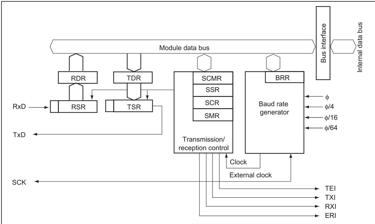
**Figure 2 Block Diagram of Synchronous Serial Data Transmission**
