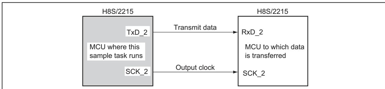
**Figure 1 Serial Data Transmission in Synchronous Mode**
