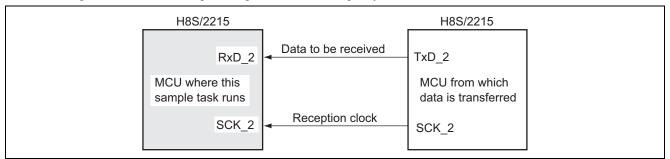
Figure 1 Serial Data Reception in Synchronous Mode
