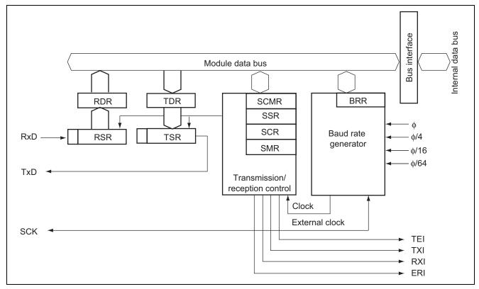
Figure 2 Block Diagram of Synchronous Serial Data Reception
