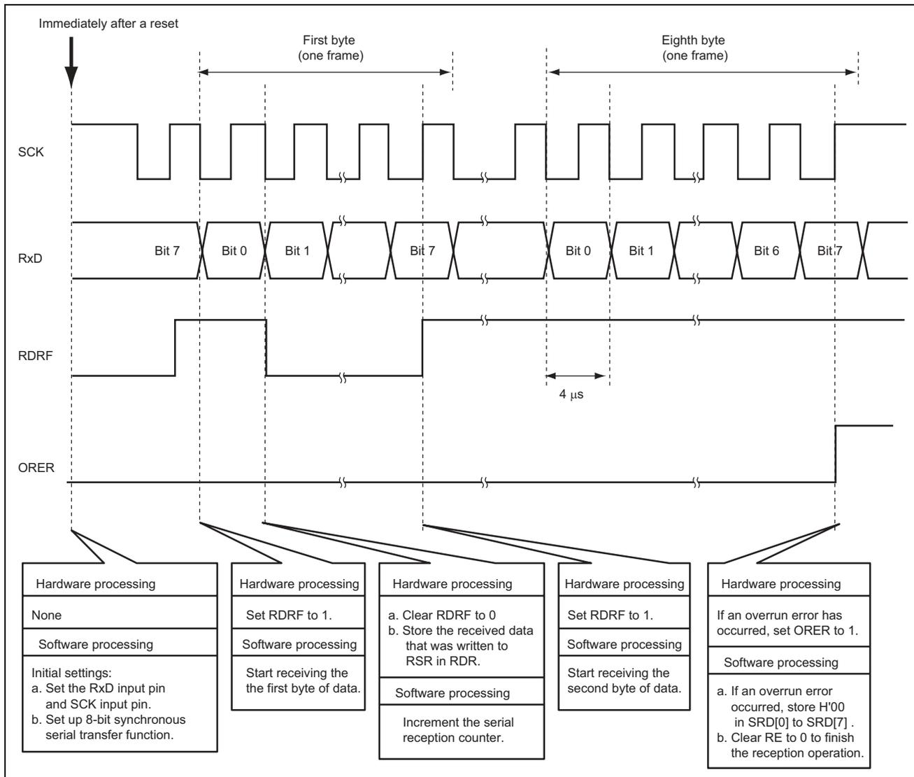
Figure 3 Operation of Serial Data Reception in Synchronous Mode
