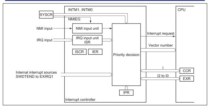
Figure 2 Block Diagram of Interrupt Controller
