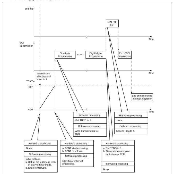
Figure 3.1 Setting end\_flg by Multiple-Interrupt Handling
