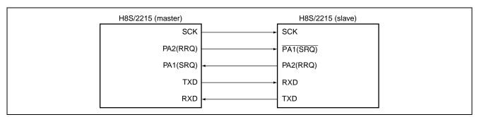
Figure 1 Block Diagram of Clock Synchronous SCI by H8S/2215
