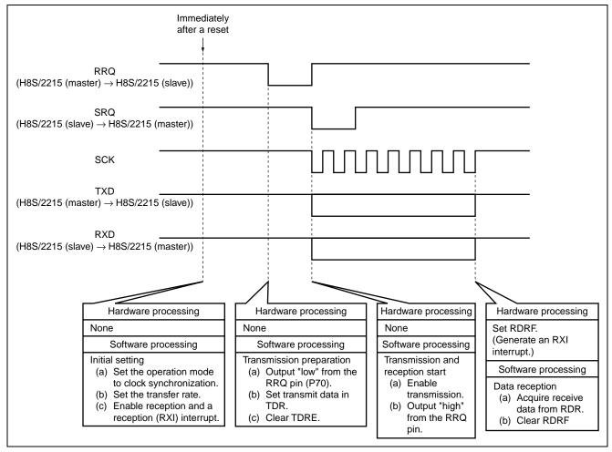
Figure 3 Principles of Operations Used for Duplex Transmission
