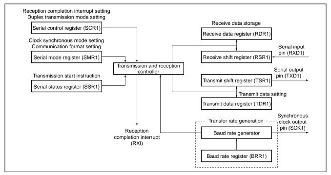
Figure 2 SCI Block Diagram
