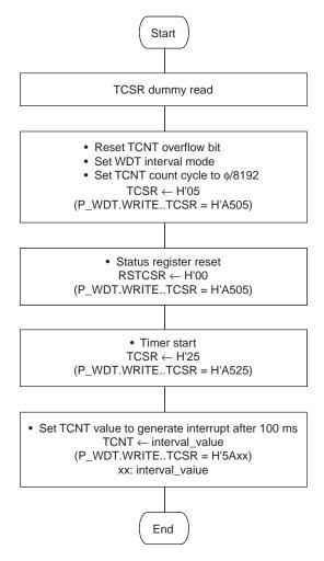
Note: As WDT related registers have a hardware reset operation function, there is a specific writing procedure. See the hardware manual for details.
