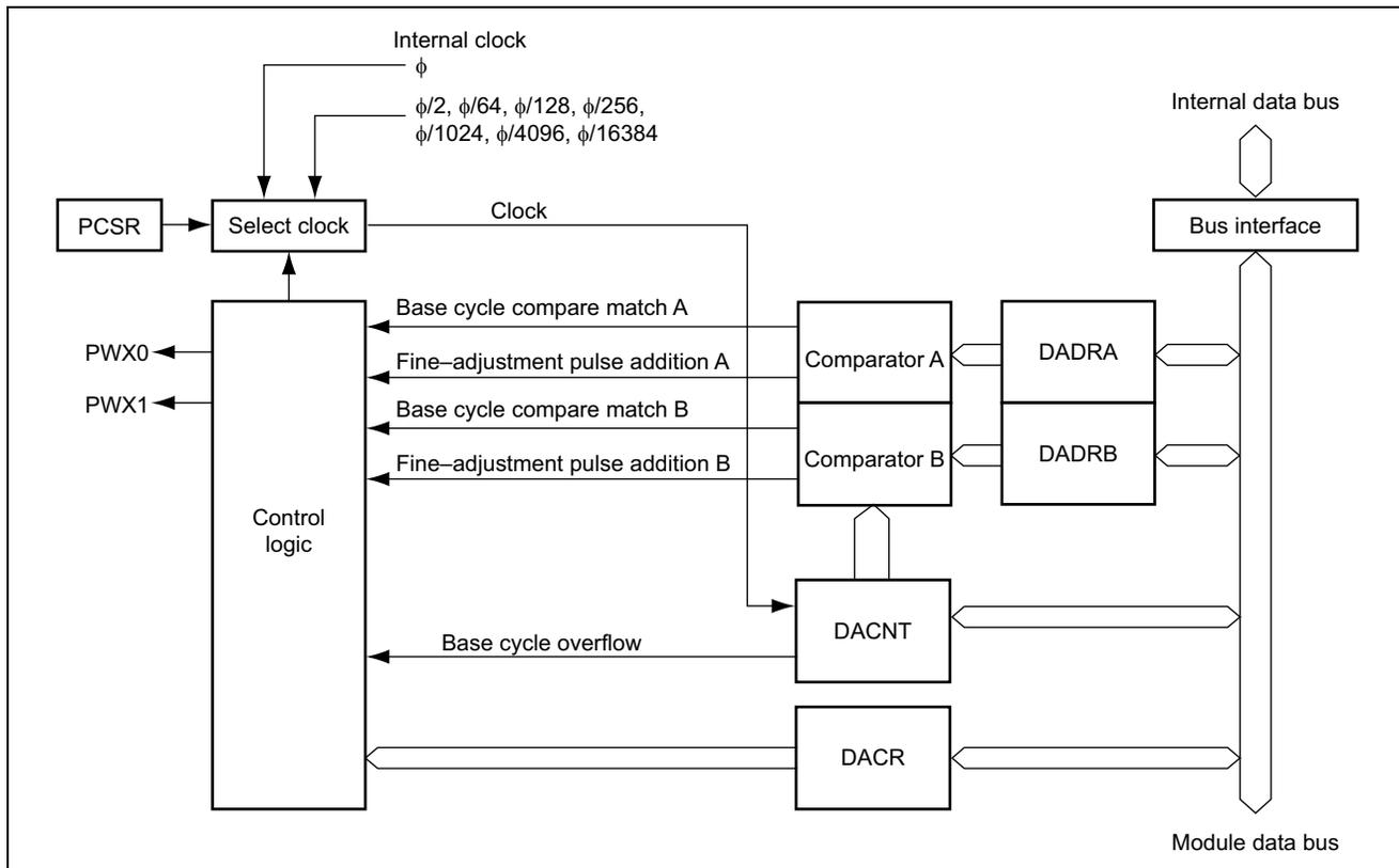
**Figure 2 Block Diagram of 14-bit PWM Module**
