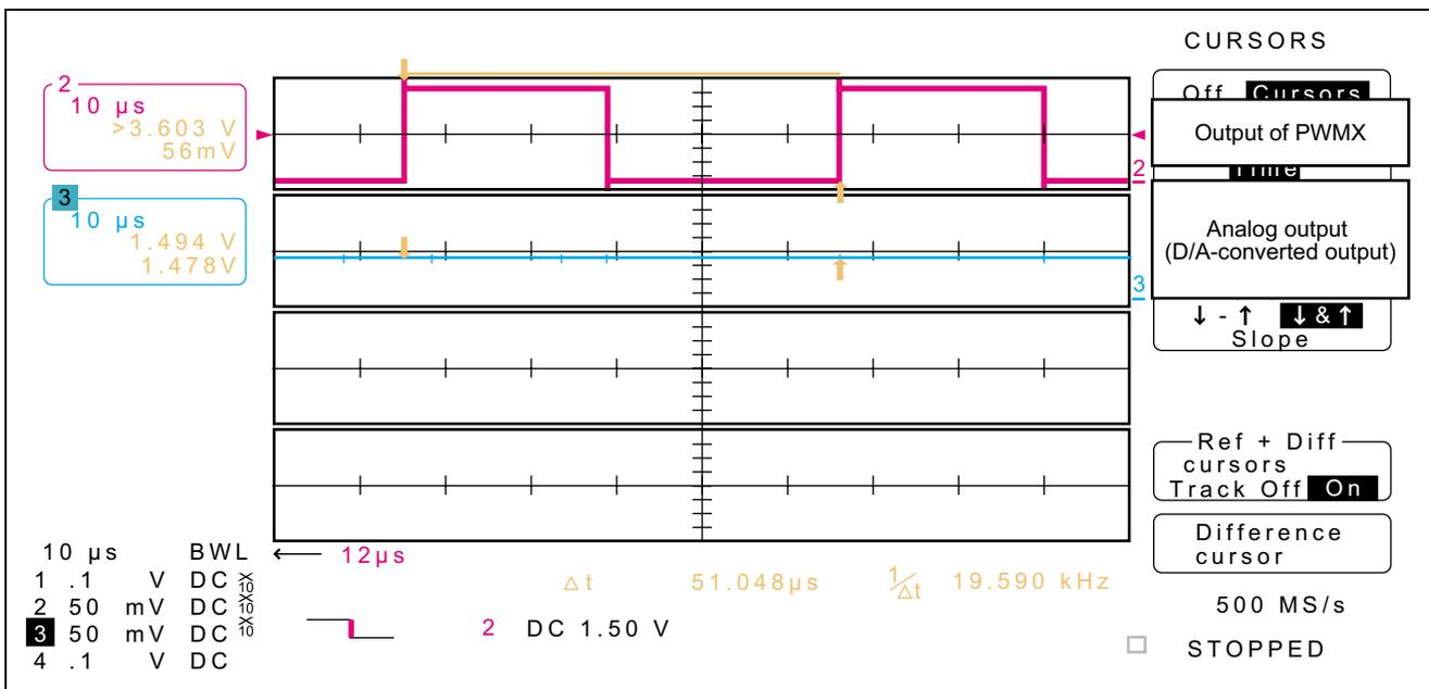
**Figure 4 D/A-Converted Waveform Generated by Using the 14-bit PWM Function (for Reference)**
