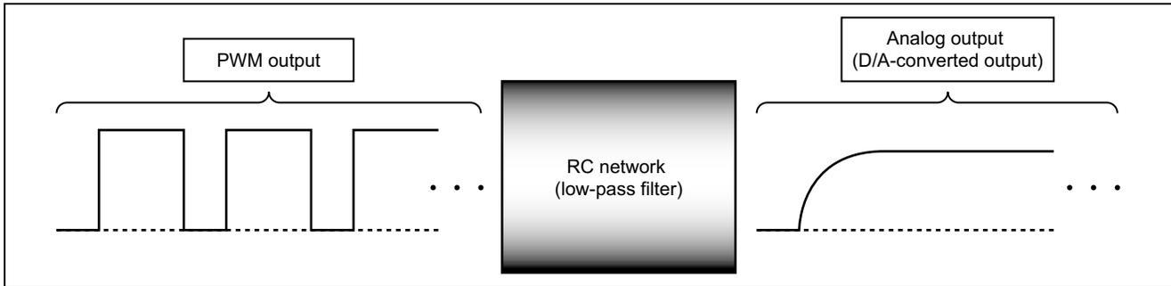
**Figure 3 Operation of a D/A Converter Driven by the 14-bit PWM Function**
