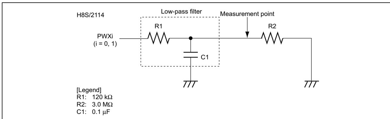
**Figure 1 Example Circuit for Use as a D/A Converter**
