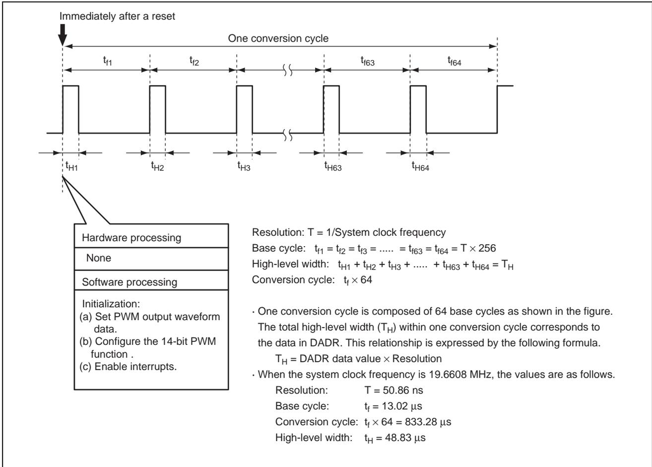
Figure 3 Operation of Duty Cycle-Controlled Pulse Output by Using 14-bit PWM Function
