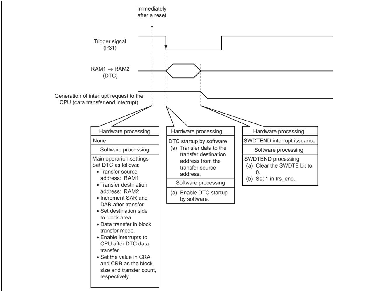
Figure 3 Principles of Operations Used for Data Transfer Started up by Software
