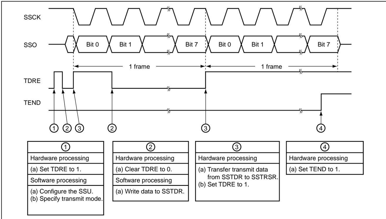
Figure 3 Operation Timing in Transmit Mode
