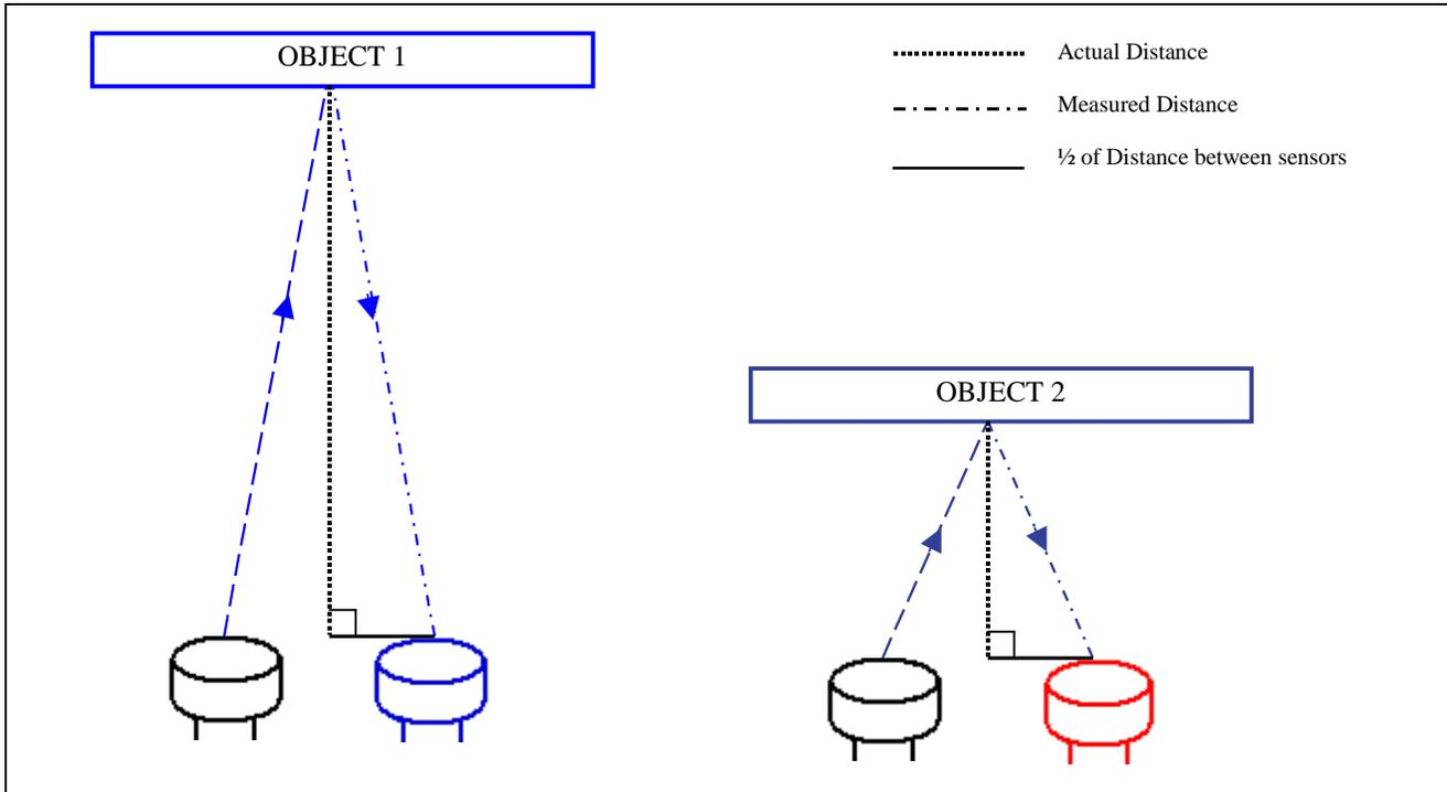
**Figure 10 Illustration of Actual Distance Measured**
