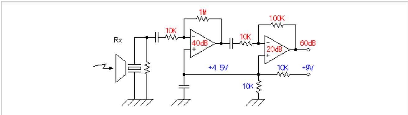
Figure 4 Signal Amplification Circuit
