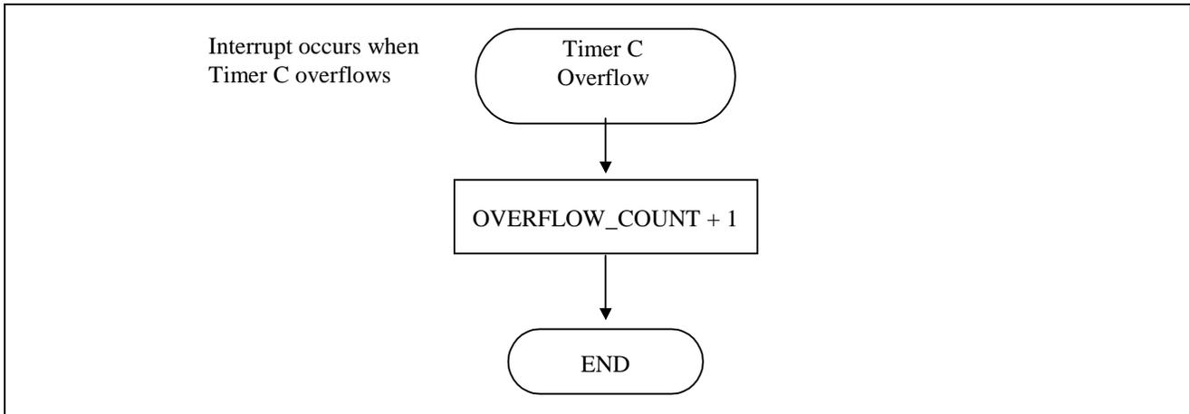
Figure 12 Timer C Overflow Interrupt Service Routine
