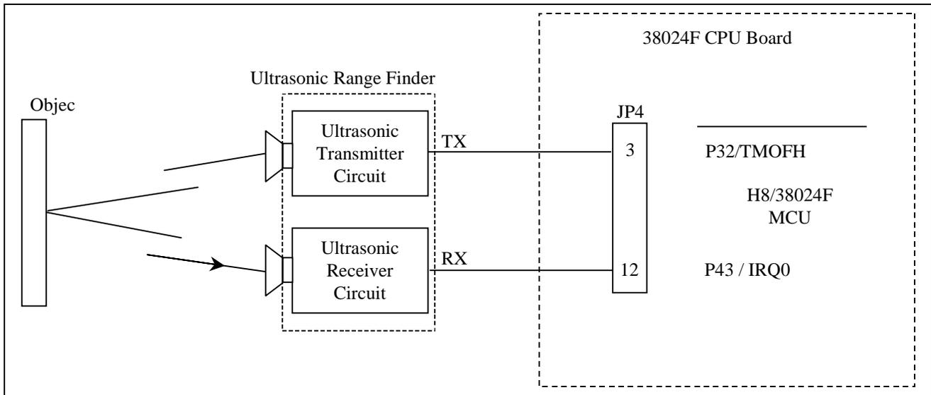
**Figure 6 Microcontroller Setup with Ultrasonic Range Finder**
