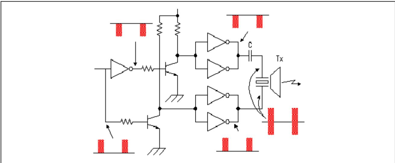
Figure 3 Transmitter Circuit
