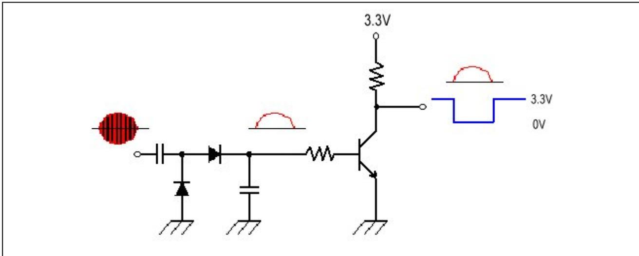
**Figure 5 Signal Detection Circuit**
