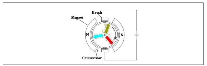
Block Diagram of Permanent Magnet DC Motor
