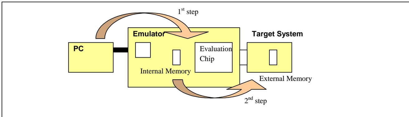
If the downloaded area is within the emulator (internal memory), the speed will be fast. However if the downloaded area is at external target area, it will need to transfer the data from the PC to the emulator (internal), and through the evaluation chip, transfer the data out to the external target area. This mechanism will be further slowed down if the user configure the evaluation chip to a slow operating frequency.
