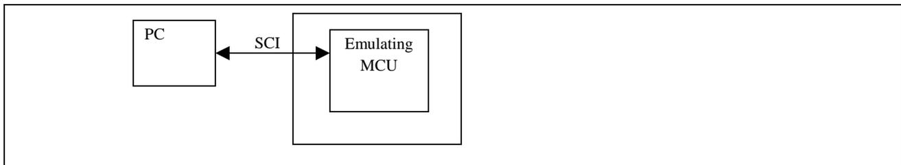
Another implementation is to directly use the emulating MCU serial port's interrupt to perform the communication. Thus user program shall not disable the interrupt, if otherwise the PC will not be able to communicate with the MCU.
