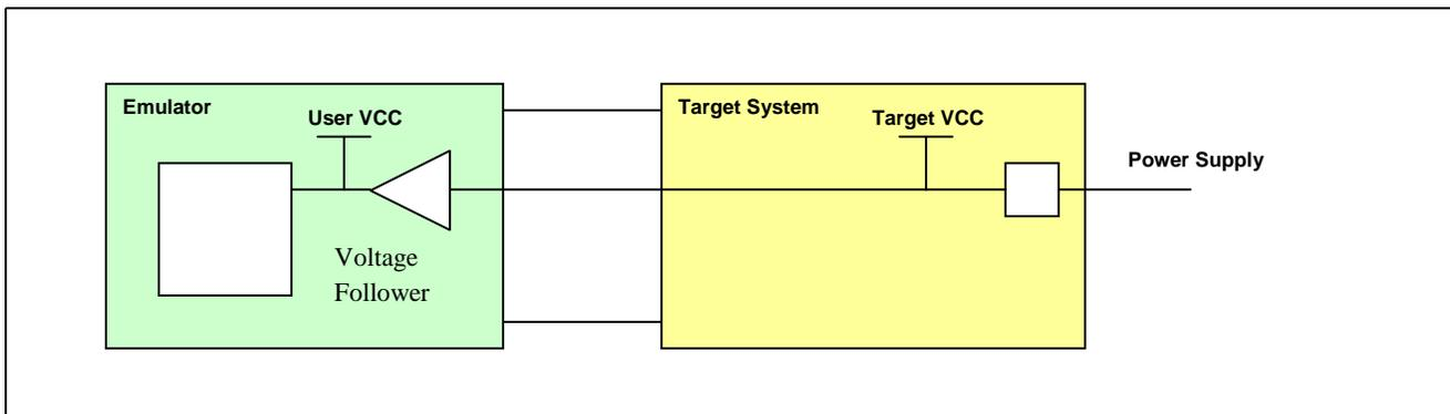
From the above diagram, Hardware developers can rest assured that the emulators will not draw current from the target. The emulator will generate an internal voltage (User Vcc) for internal operation, which is based on a target system supply (Target Vcc). When current measurement is made on the target, developers will have to take into the account that the emulating MCU is not consuming the target power.
