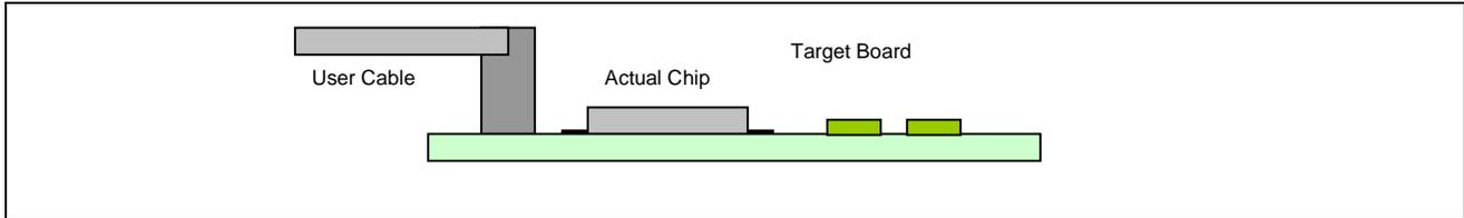
Emulator connection to a target system is via a dedicated user system interface cable.
