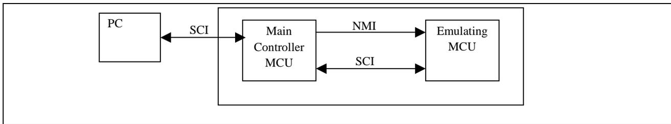
One example is to use another MCU to be the master controller to communicate with the PC, and generate a NMI interrupt to the emulating CPU. In this design, the NMI of the emulating CPU is used (The serial port of the emulating MCU is used to obtain command & data from the PC).
