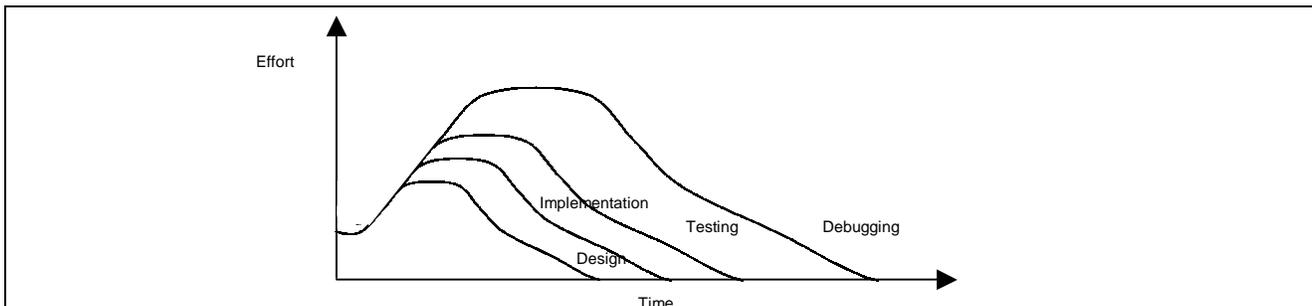
The implementation stage always takes shorter time to complete than the integration stage. The integration stage took up longer hours because this is the stage whereby most bugs are discovered. Statistic showed that with a clean compile, there is one bug detected per 20 lines of code written. i.e., a 32-k code will produce an approximate 1500 errors of code.
