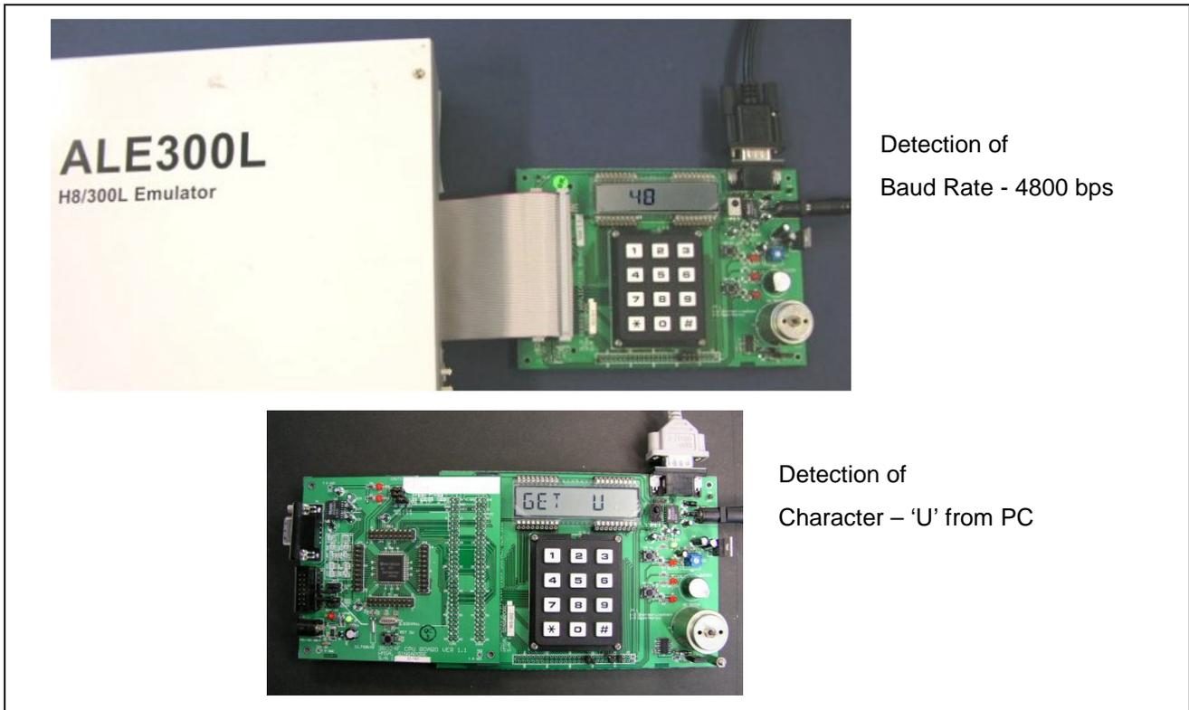
**Figure 2 Use of ALE300L Emulator or the SLP CPU Board with the General Application Board**
