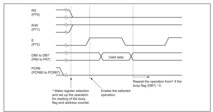
Figure 3 Reading of Busy Flag (DB7) and Address Counter (DB0 to DB6)
