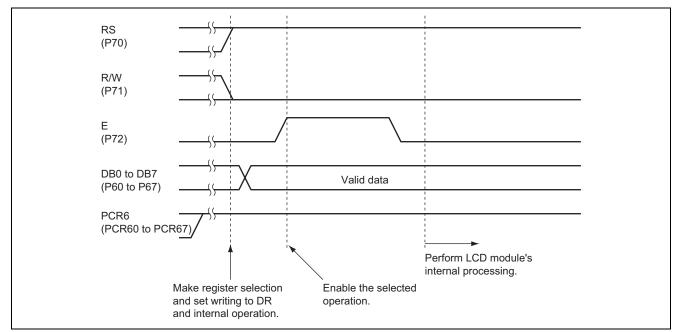
Figure 4 IR Write and Internal Operation (DR  $\rightarrow$  DD RAM or CG RAM)
