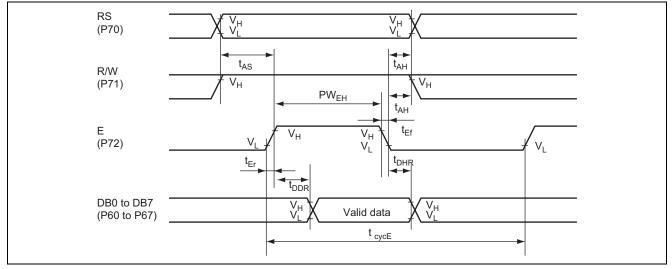
Figure 8 Bus Read Operation Sequence
