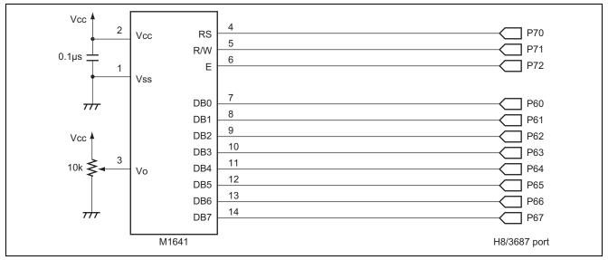
An LCD is connected as shown in figure 1 and characters are displayed on the LCD through port operation.
