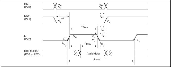
Figure 7 Bus Write Operation Sequence
