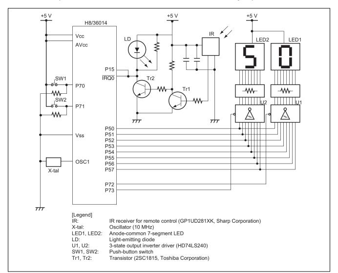
Figure 1 Hardware Configuration
