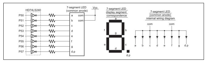
Figure 7 7-Segment LED Connection and Internal Wiring
