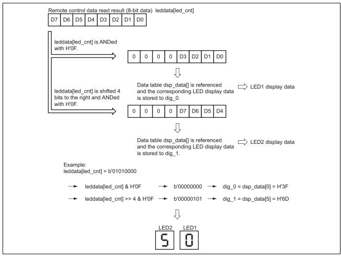
Figure 5 How Remote Control Input Data are Displayed on the LEDs
