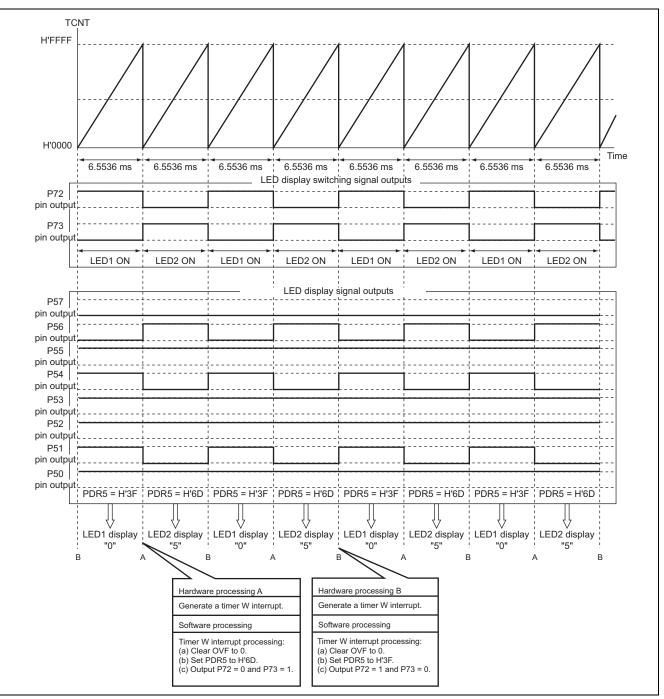
Figure 9 Principles of Operation: 7-Segment LED Display Control
