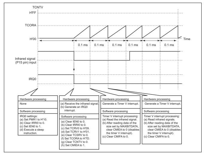
Figure 8 Principles of Operation: Remote Control Signal Reception Using Timer V
