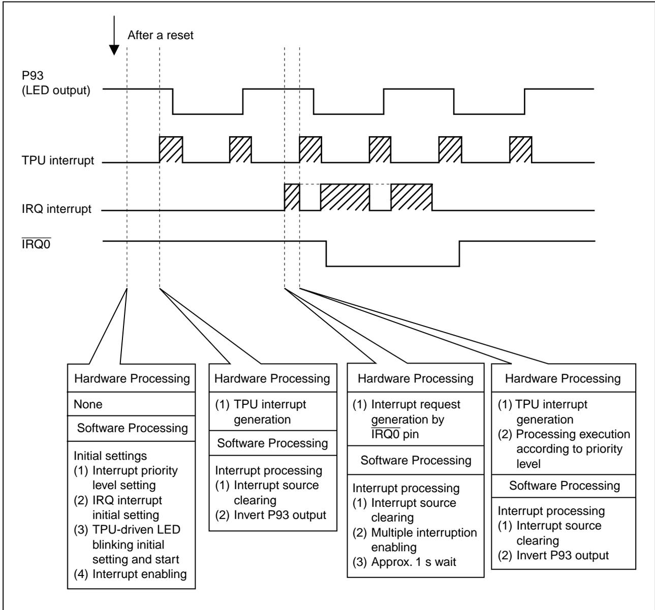
Figure 3 Principles of Operation
