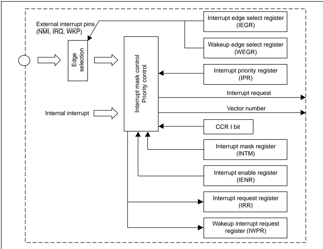
Figure 2 Block Diagram of Interrupt Controller
