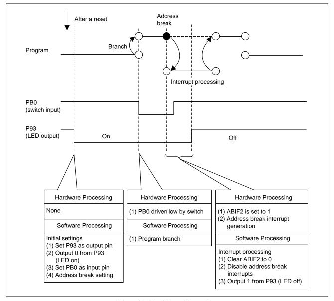
Figure 3 Principles of Operation
