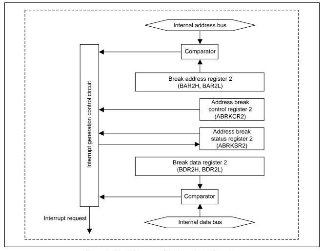
Figure 2 Block Diagram of Address Break Function
