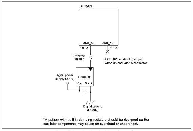
Figure 5 Example of an Oscillator Connection
