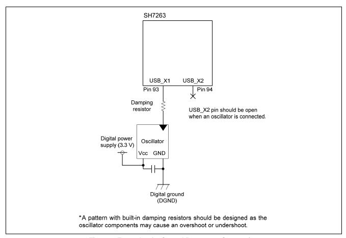
Figure 4 Example of a Crystal Resonator Connection
