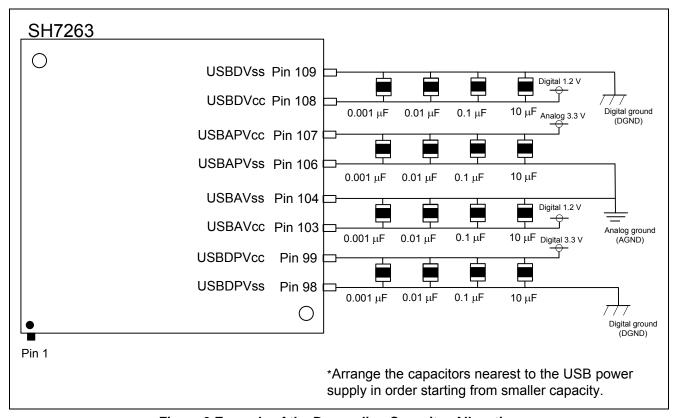
Figure 3 Example of the Decoupling Capacitor Allocation
