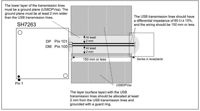
Figure 1 Design Example of the Host Controller USB Transmission Line Pattern
