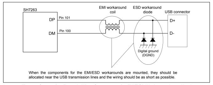
Figure 9 Connection Example When Components for EMI/ESD Workarounds are Used
