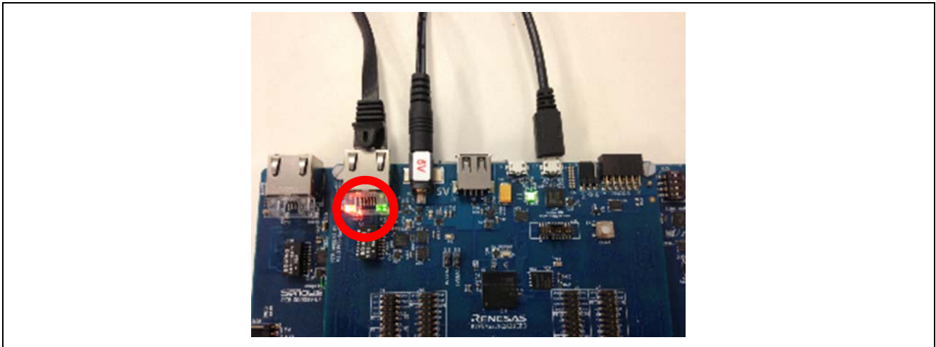
Figure 8. Orange and Green Ethernet Status LEDs
