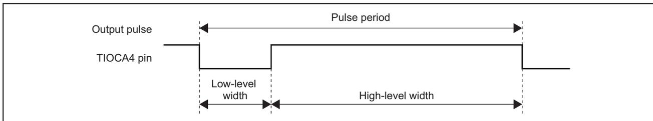
**Figure 1 Example of Long-Period Pulse Output**
