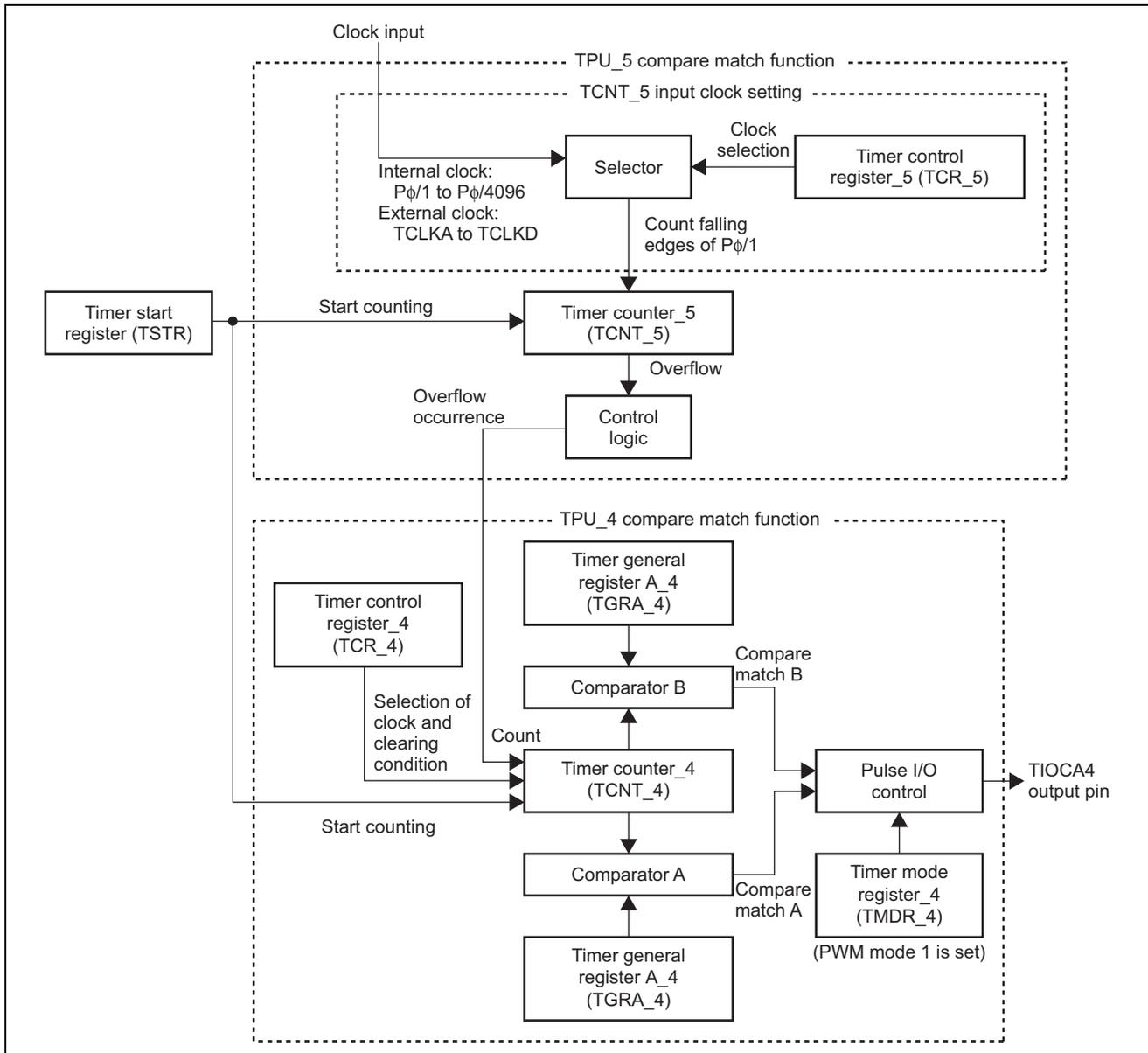
Figure 2 Block Diagram of Long-Period Pulse Output
