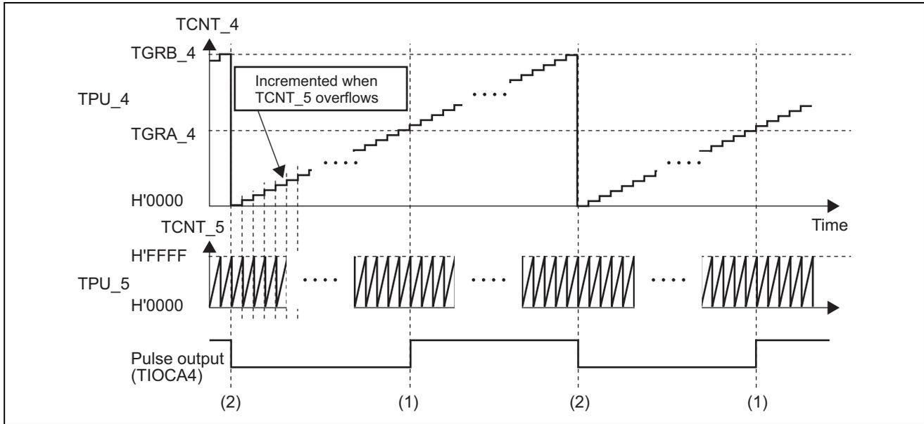
Figure 3 Operation of Long-Period Pulse Output
