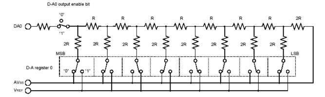
External operational amplifier should be added external before sending the signal to low impedance devices as shown below.
