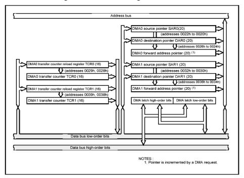
The DMA channel only accepts source <u>or</u> destination increment (not both at same time).
