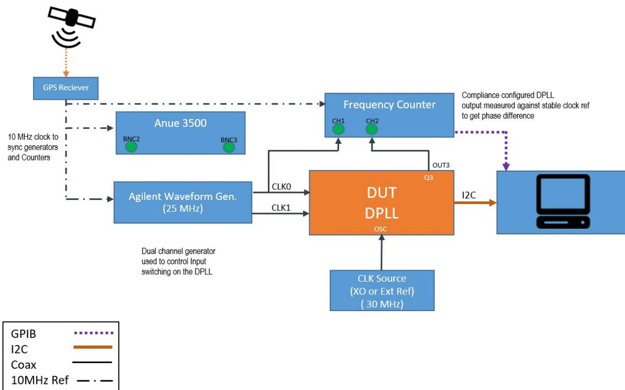
Figure 1. FemtoClock 2 SyncE Compliance Test Setup
