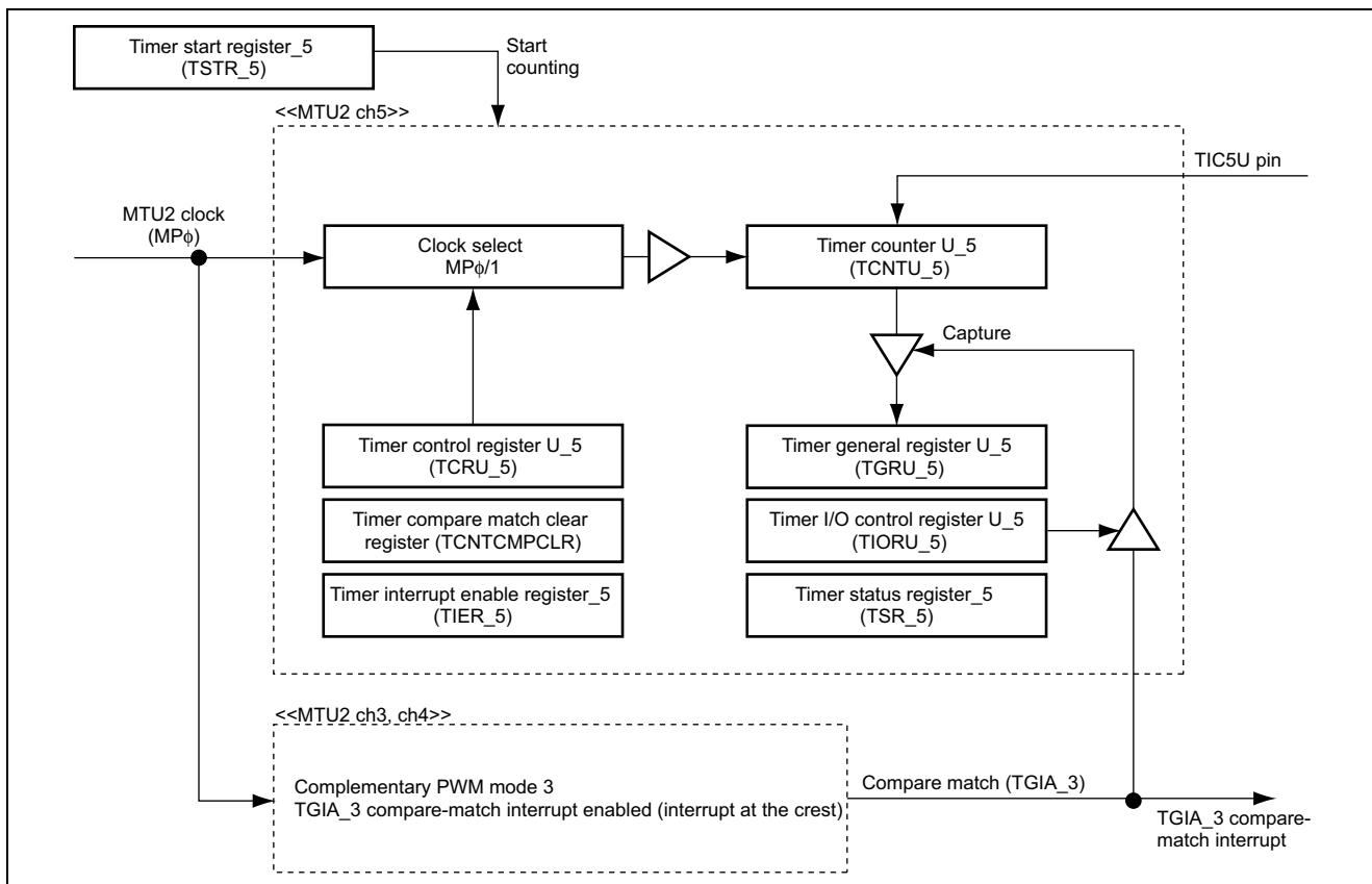
Figure 2 Block Diagram of Channel 5 of MTU2
