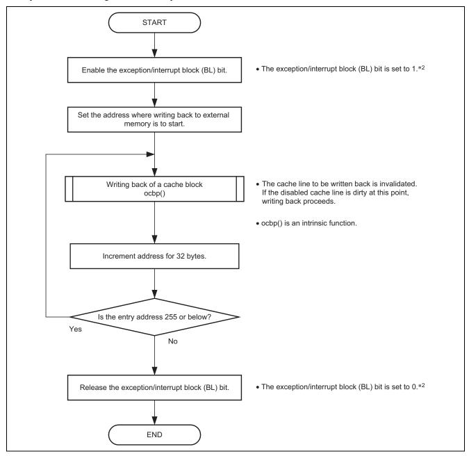
Figure 5 Procedure for Writing Back from the Operand Cache
