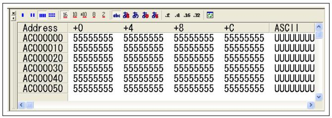
Figure 8 External Memory Area after Write-Back Operation
