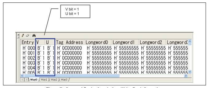
Figure 7 Operand Cache Area before Write-Back Operation
