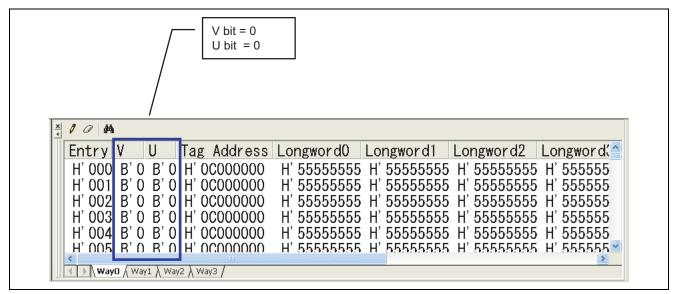
Figure 9 Operand Cache Area after Write-Back Operation
