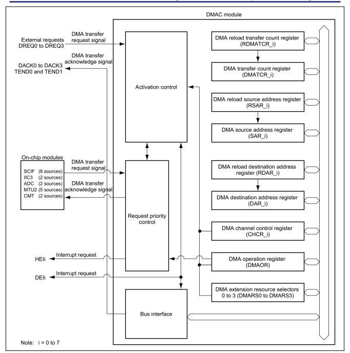
Figure 1 Schematic View of the DMAC
