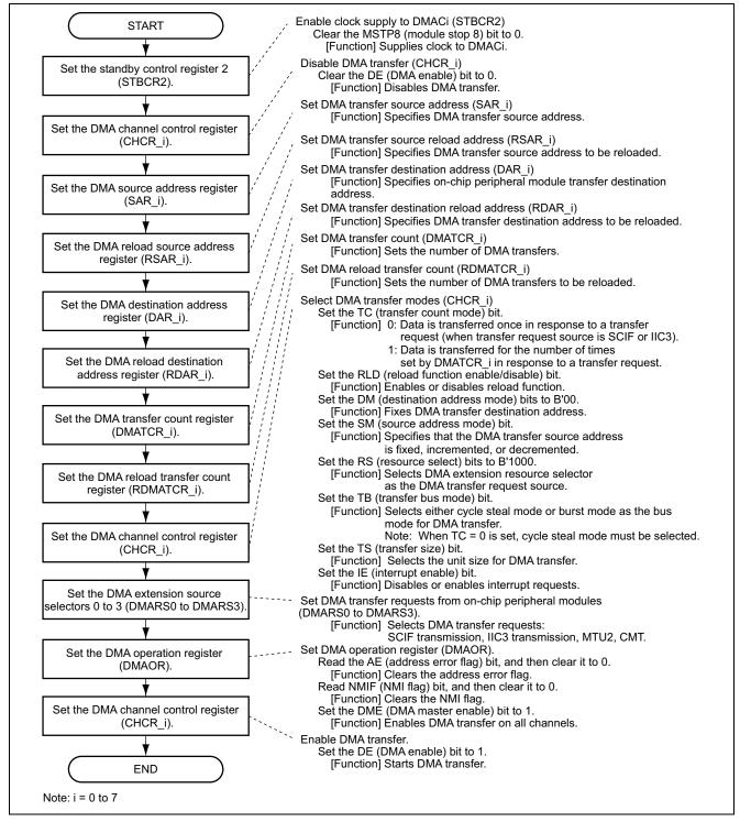
Figure 2 Example Flow for Initial Settings of the DMAC
