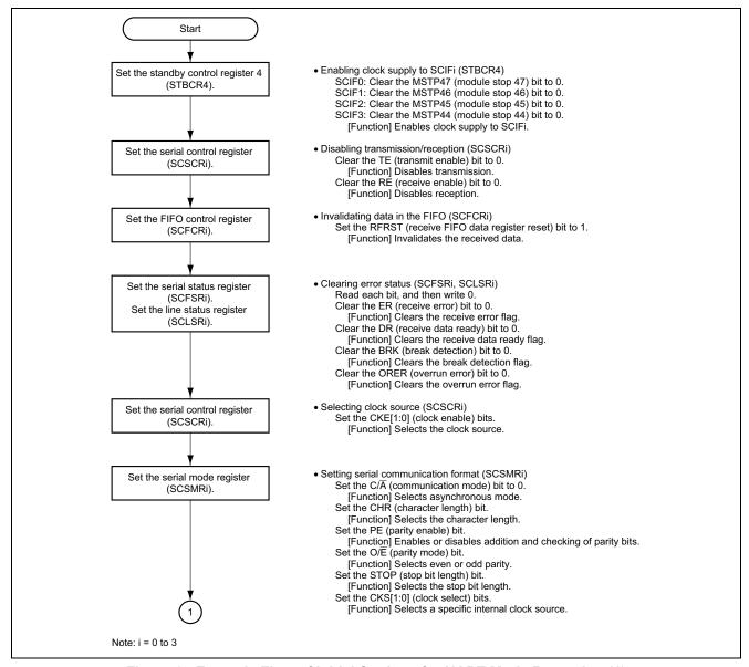
Figure 2 Example Flow of Initial Settings for UART Mode Reception (1)
