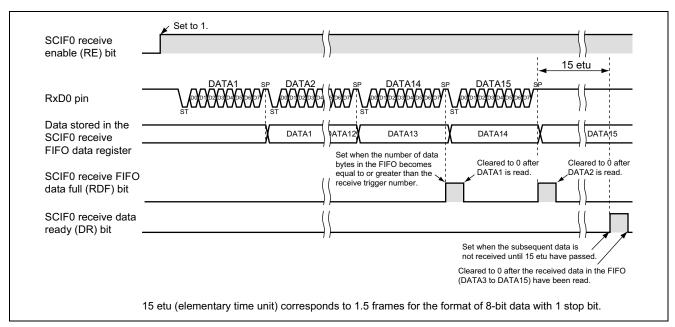
Figure 5 Timing of Sample Program Operation
