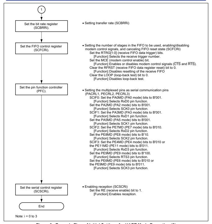
Figure 3 Example Flow of Initial Settings for UART Mode Reception (2)
