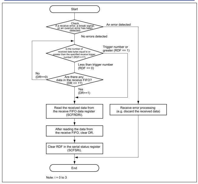
Figure 4 Example Flow of UART Mode Reception Processing
