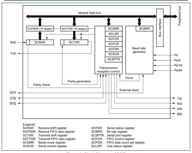
Figure 1 Block Diagram of SCIF
