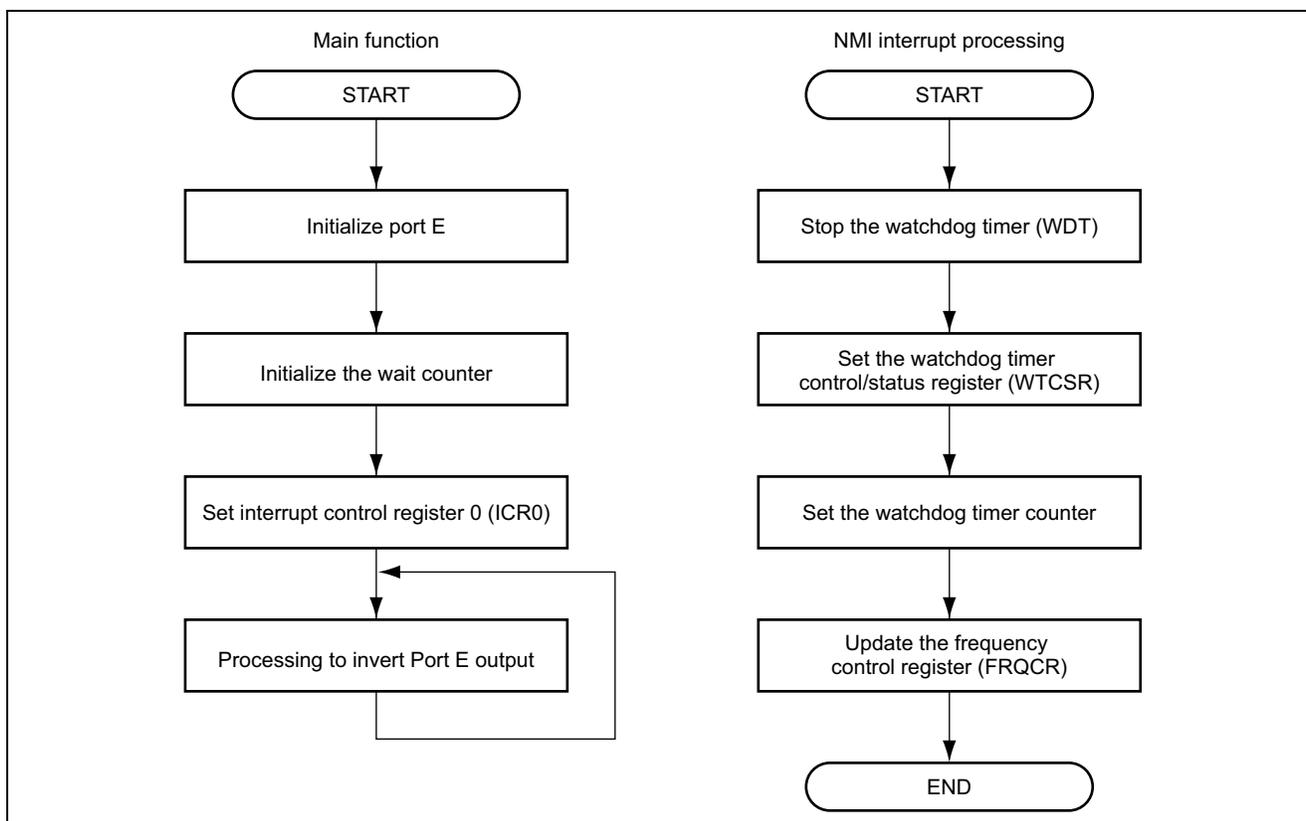
**Figure 5 Flow of Processing by the Sample Program**
