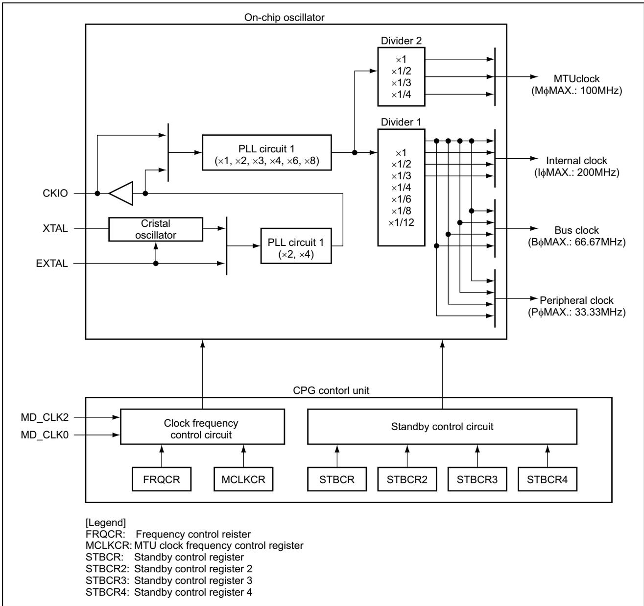
Figure 1 Schematic View of the CPG
