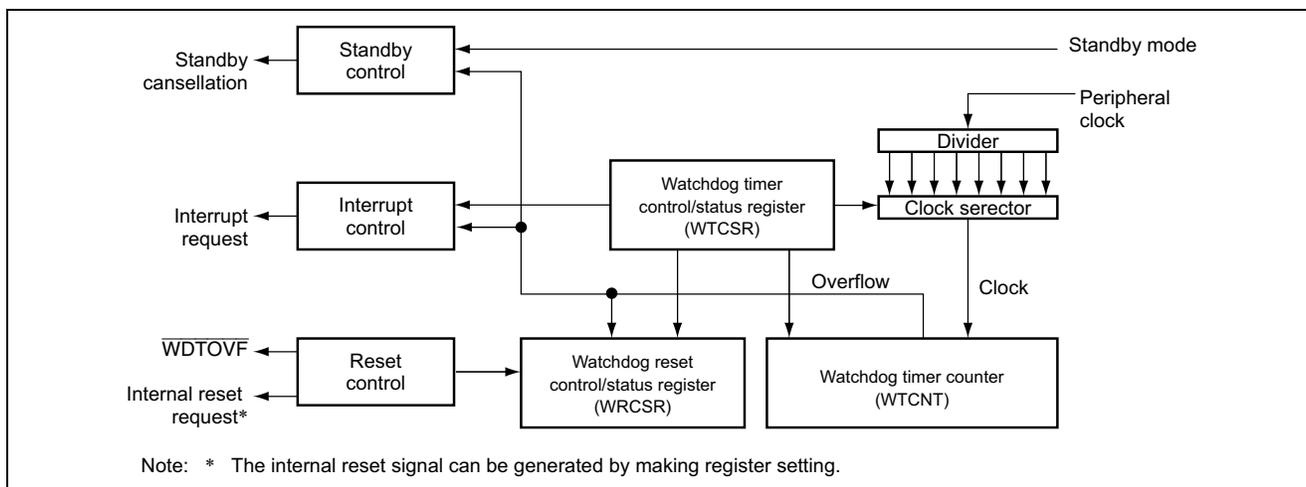
Figure 2 Schematic View of the WDT
