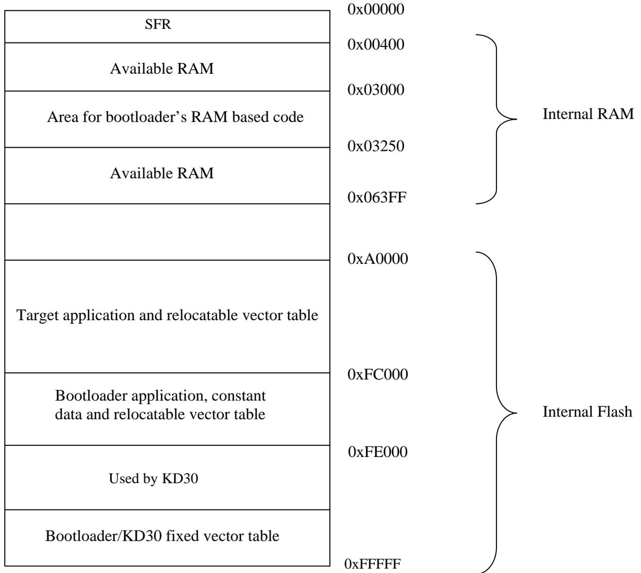
Figure 3: Bootloader and Target Application Memory Map
