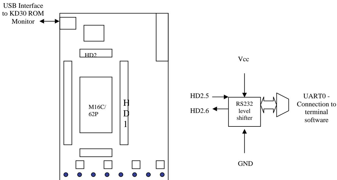
Figure 1: M16C/62P 3-D Kit Based System Block Diagram
