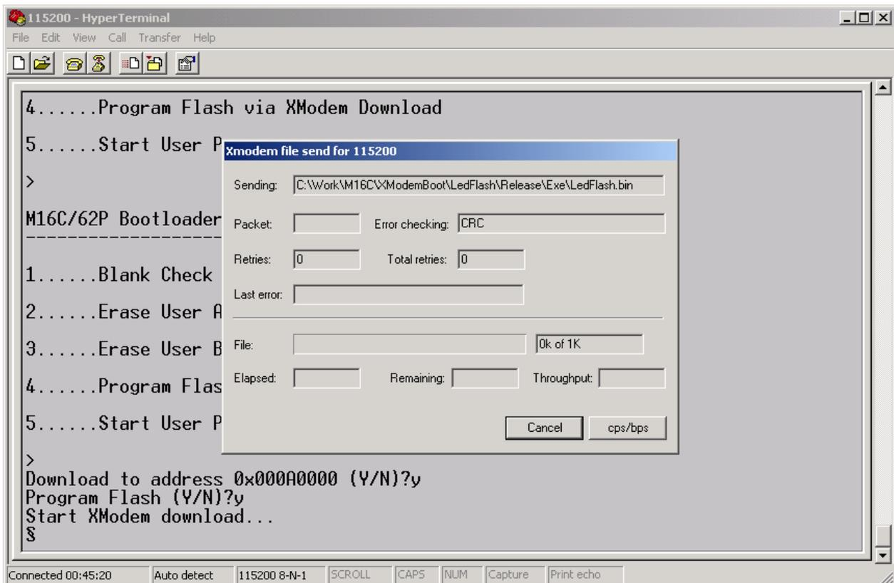
Figure 11: Downloading the Target Application Using XModem
