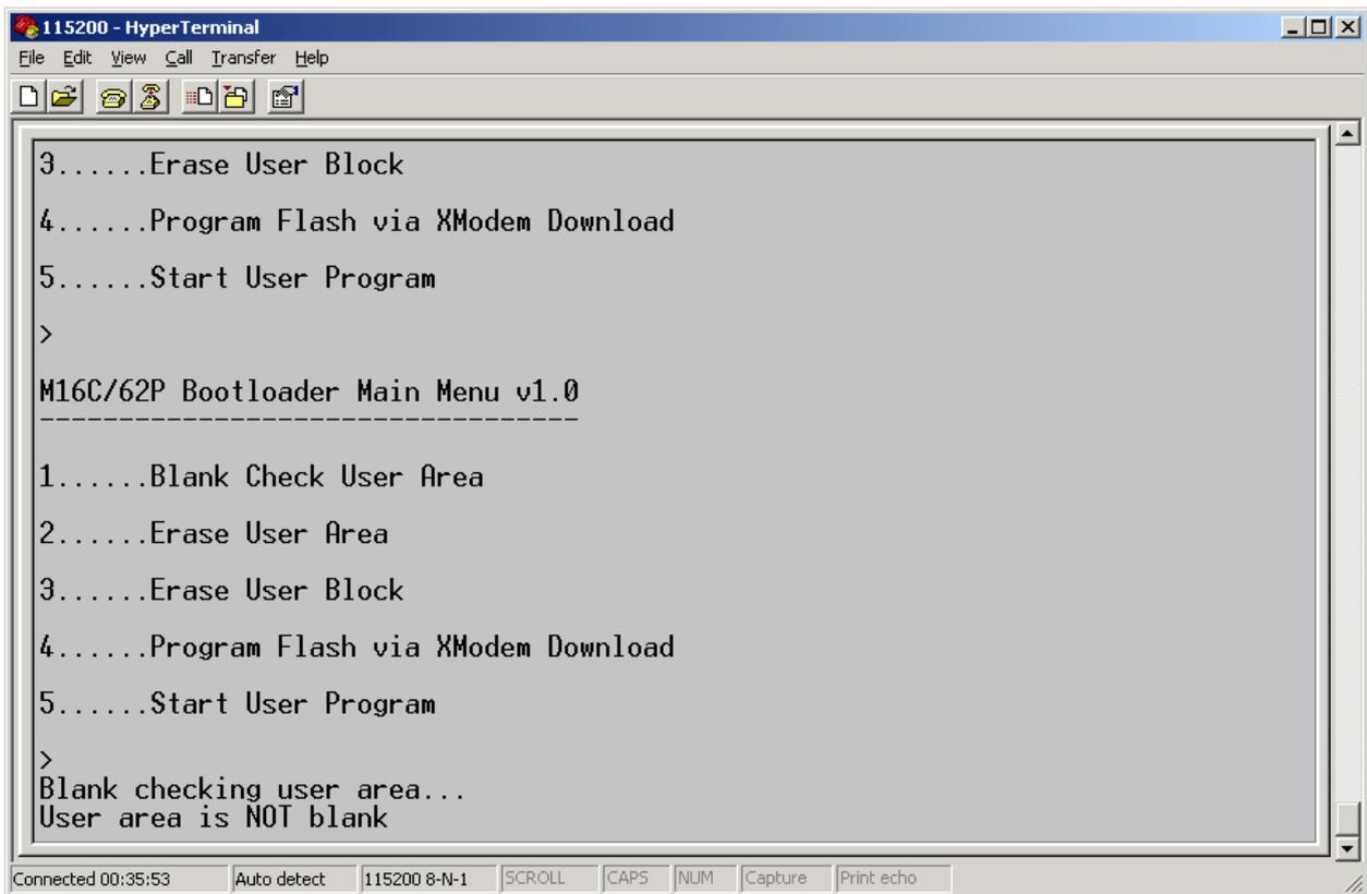
Figure 9: Blank Checking the User Area
