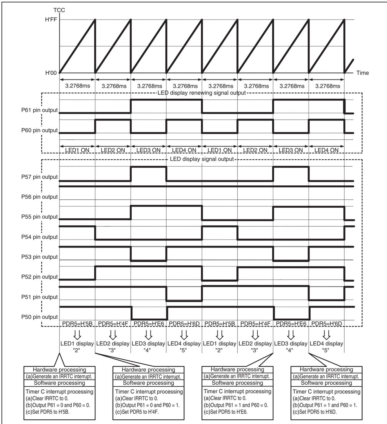
Figure 9 Description of 7-Segment LED Display Control
