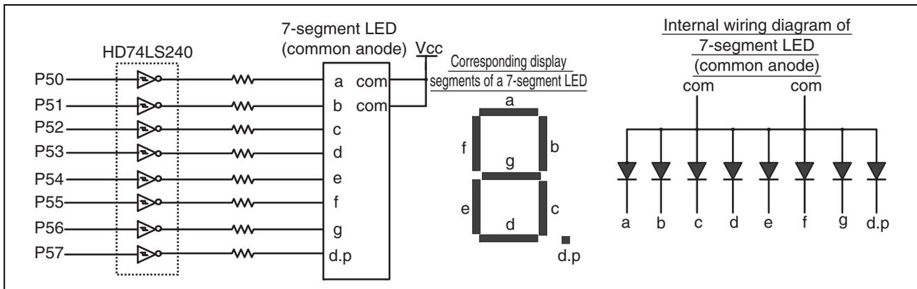
**Figure 7 Connection Diagram and Internal Connections of 7-Segment LED**
