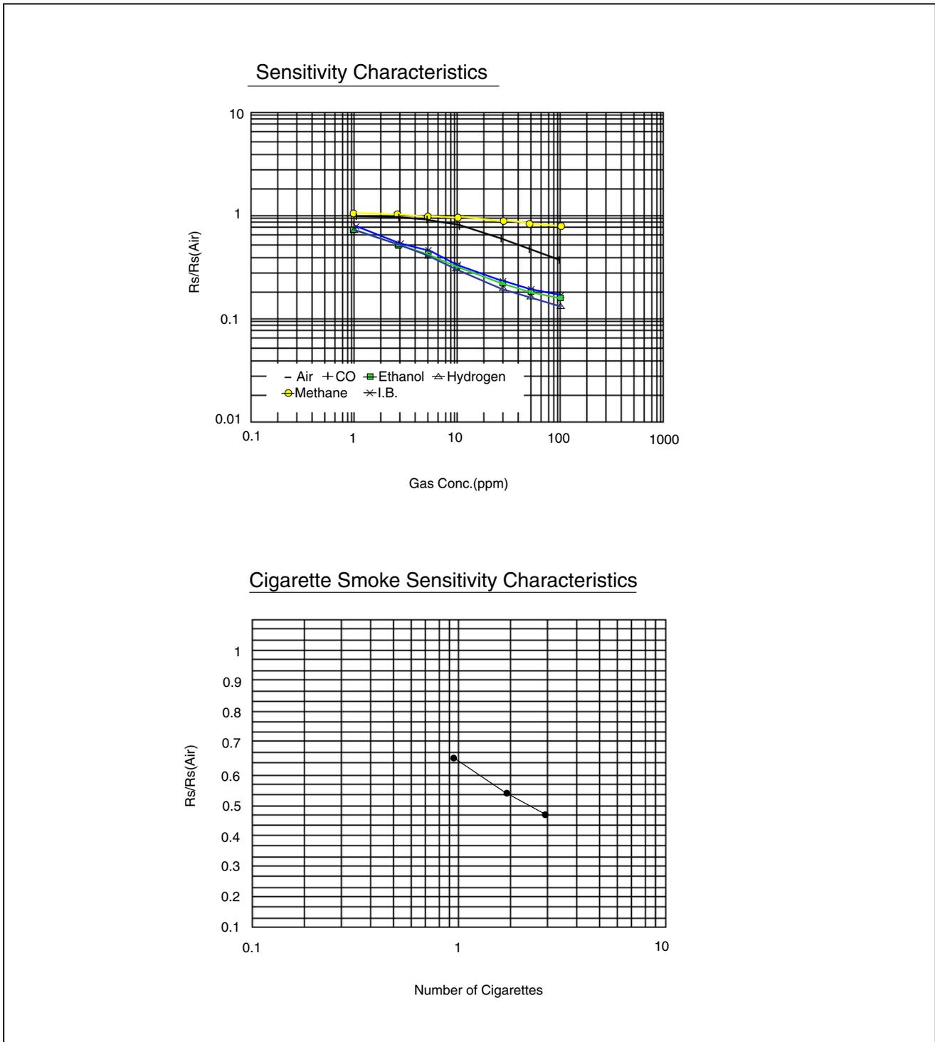
**Figure 3 Sensor Sensitivity Characteristics (Reference Values)**
