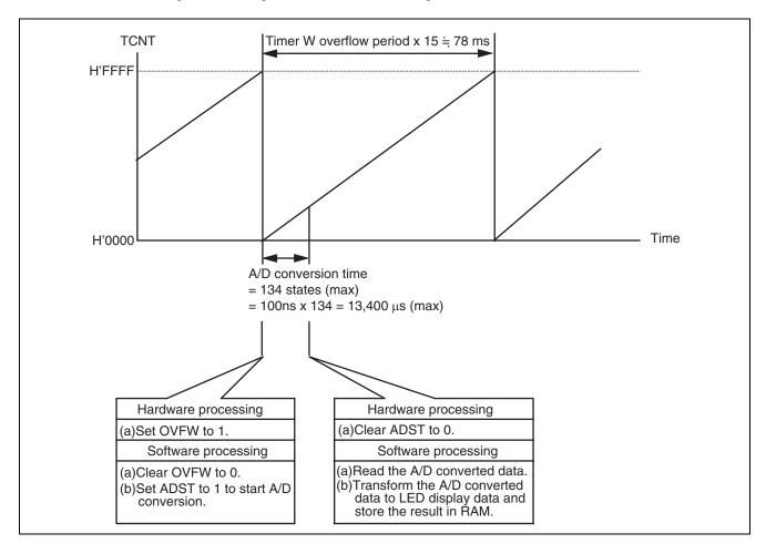
Figure 7 A/D Conversion of the AN0 Pin Signal when Timer W is Used
