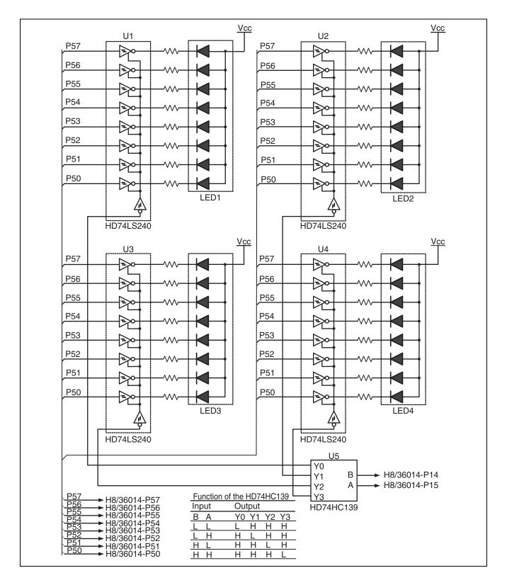
Figure 3 Control of 7-Segment LEDs
