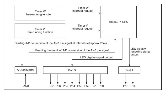
Figure 5 Block Diagram of Functions Used in This Sample Task
