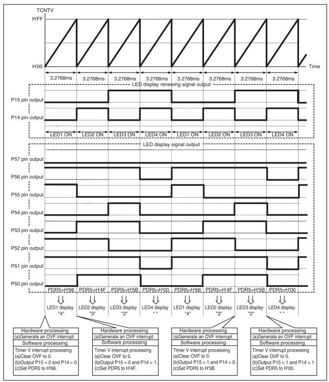
Figure 8 Description of 7-Segment LED Display Control
