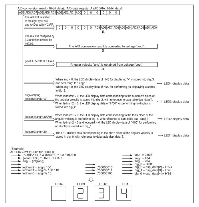
Figure 4 Display of Angular Velocity on the LEDs
