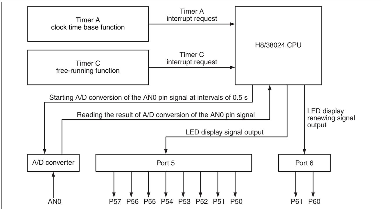
**Figure 5 Block Diagram of Functions Used in This Sample Task**
