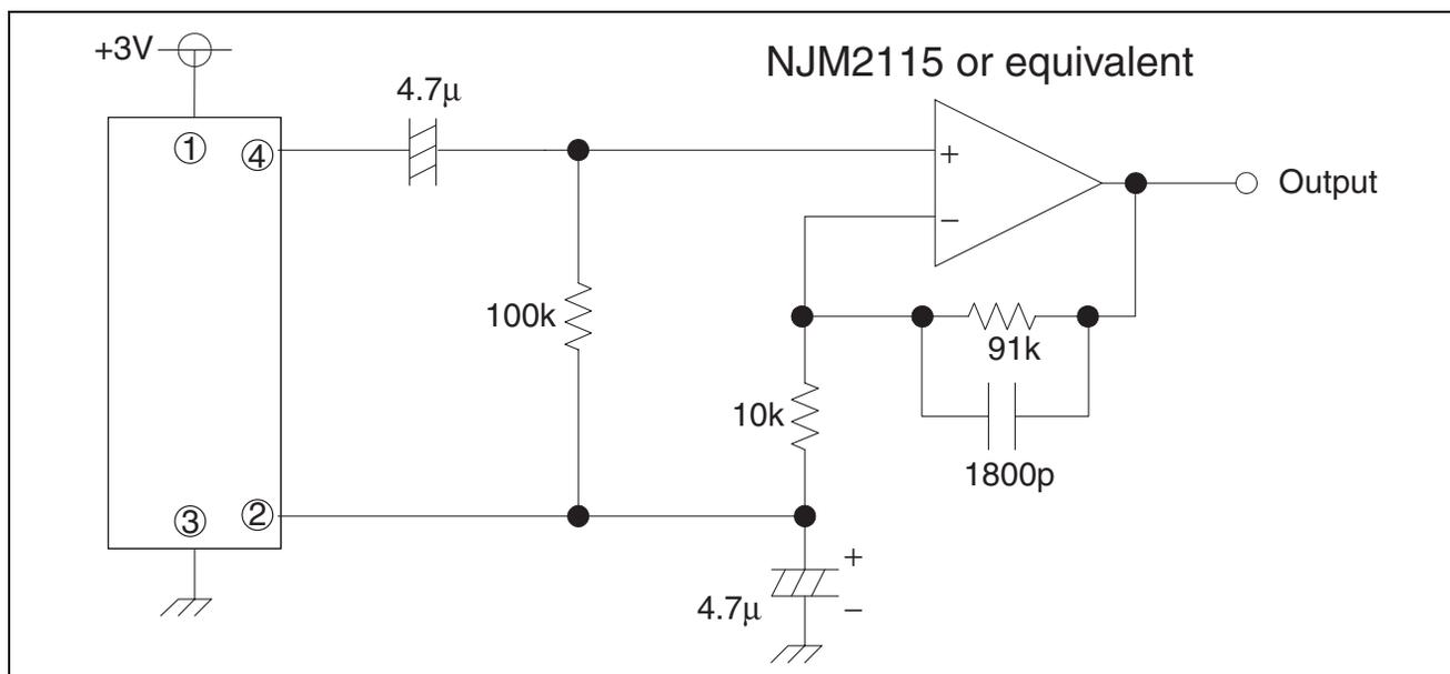
**Figure 2 Sensor Standard Amplification Circuit (Sample Circuit)**
