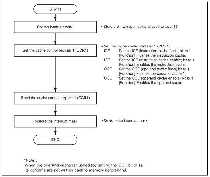
Figure 2 Example Flow for Settings Up the Cache
