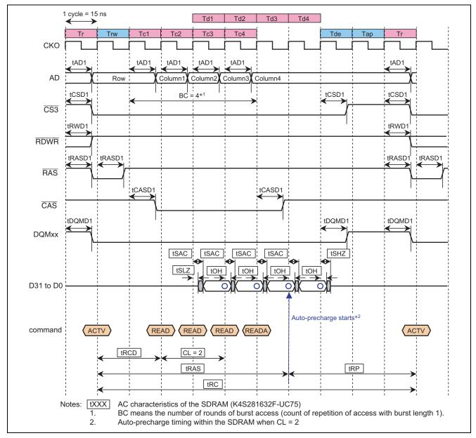
Figure 6 Timing for Burst Reading of the SDRAM
