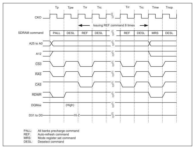
Figure 4 Example of Timing in Writing to the SDRAM Mode Register
