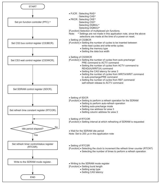
Figure 3 Example of Procedure for Initial Settings to Place SDRAM in the CS3 Space
