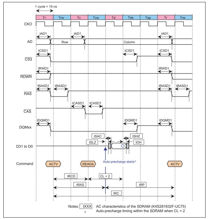
Figure 5 Timing for Single Reading of the SDRAM
