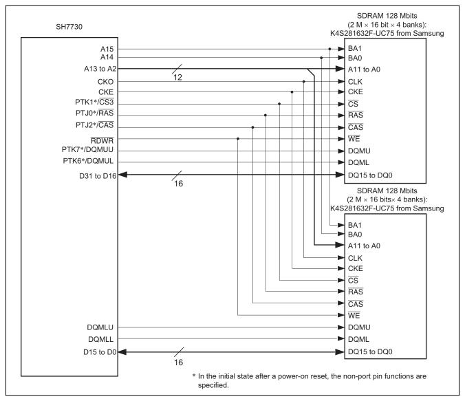
Figure 2 Example of Circuitry for SDRAM Connection (128-Mbit SDRAM × 2, 32-Bit Bus)
