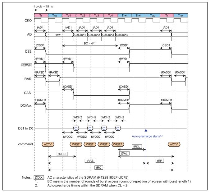
Figure 8 Timing for Burst Writing of the SDRAM
