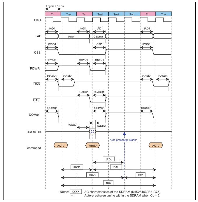
Figure 7 Timing for Single Writing of the SDRAM
