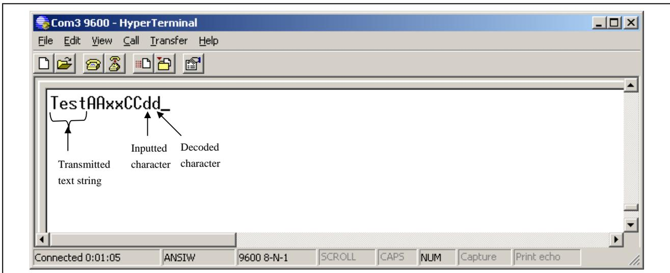
Figure 7 Results displayed on PC HyperTerminal
