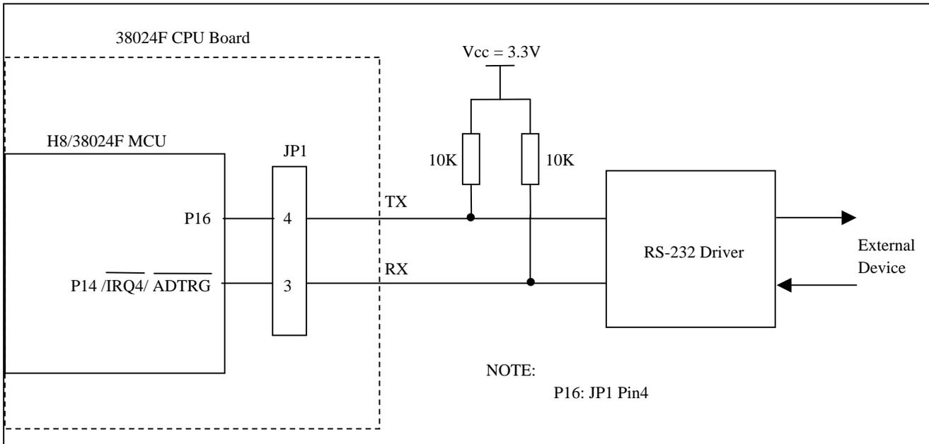
Figure 3 Micon setup with RS-232 driver
