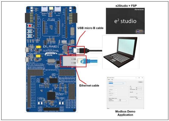
Figure 5. EK-RA8D1 Board Connection Configuration
