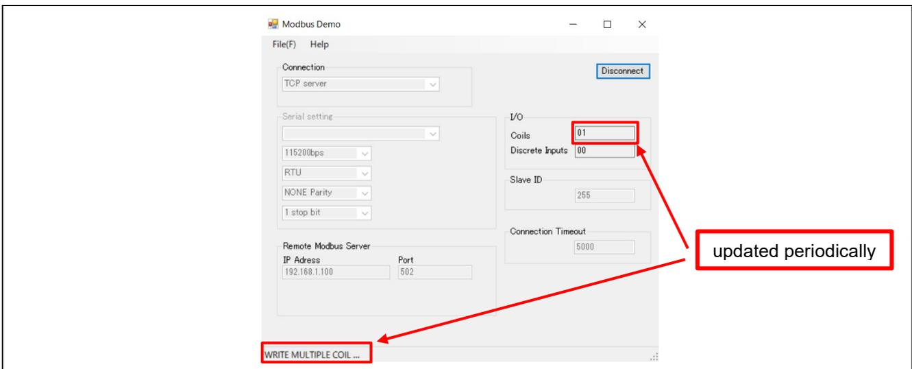
2. When SW1 is ON, LED1-3 light up depending on the input value of the coil value of the demo application's I/O.
