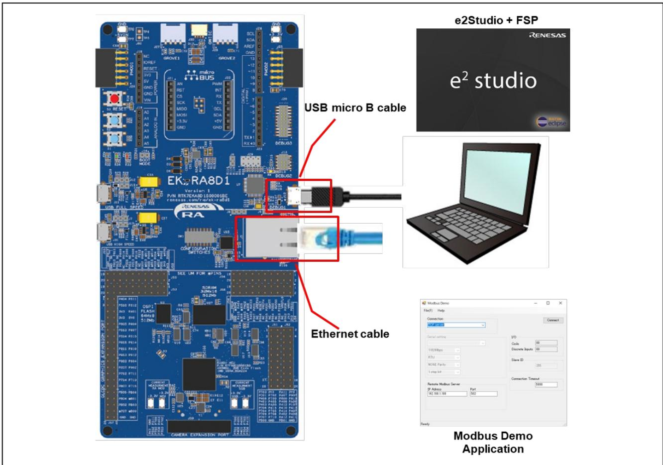
**Figure 5. EK-RA8D1 Board Connection Configuration**
