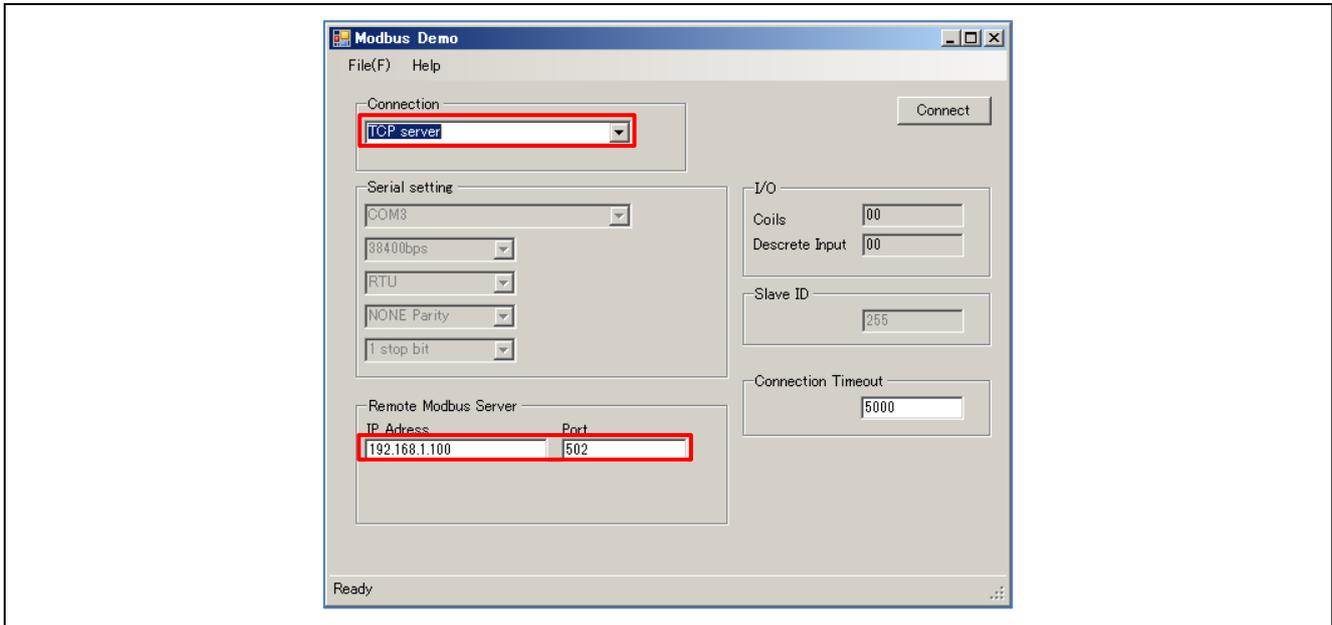
2. When **Connect** button is clicked, LED blinking is started with Modbus communication.
