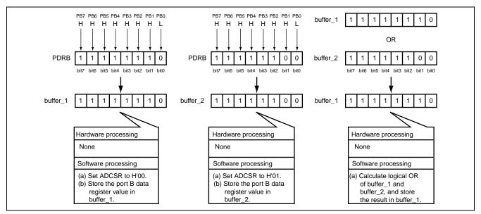
Figure 3.1 Description of Port B 8-Bit Parallel Input Operation
