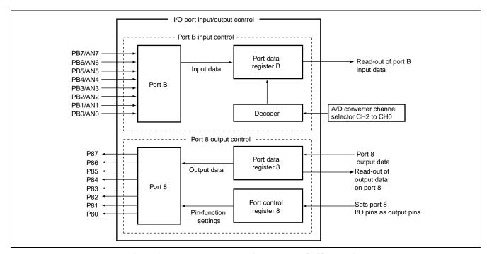
Figure 2.1 Port B Input Function and Port 8 I/O Function
