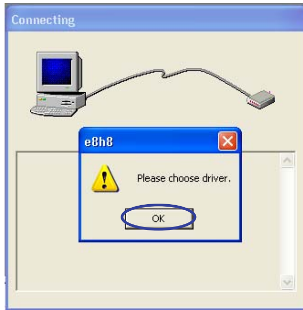
Figure 6.13 Prompt to Choose the Driver for the First-Time Connection of E8 Emulator through USB
