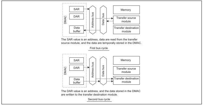
Figure 1 Flow of Data in Dual Address Mode
