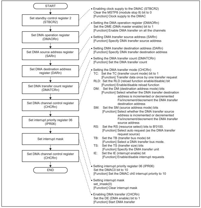
Figure 3 Flowchart of DMAC Initialization
