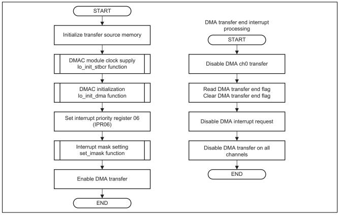
Figure 5 Flowchart of Processing by the Sample Program
