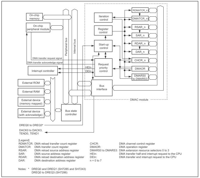
Figure 2 Block Diagram of the DMAC
