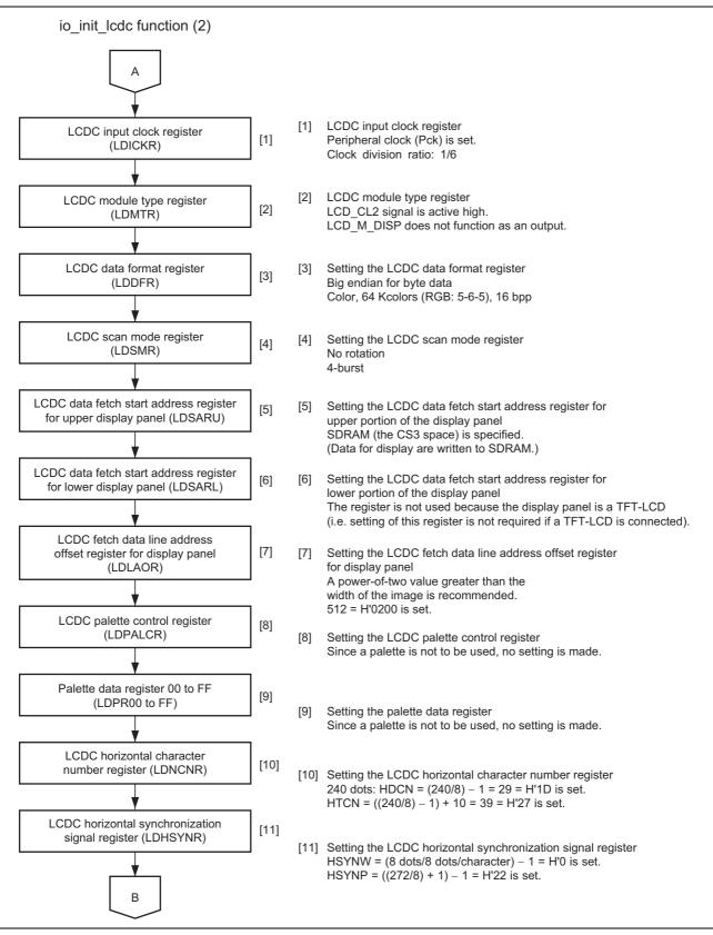
Figure 12 Flow for Initialization of the LCDC (2)
