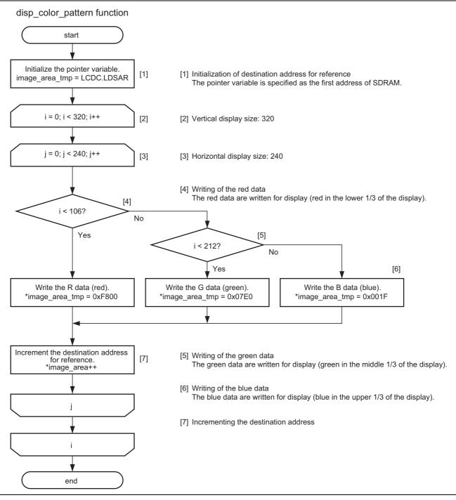
Figure 14 Flow for the Setting the Color Patterns
