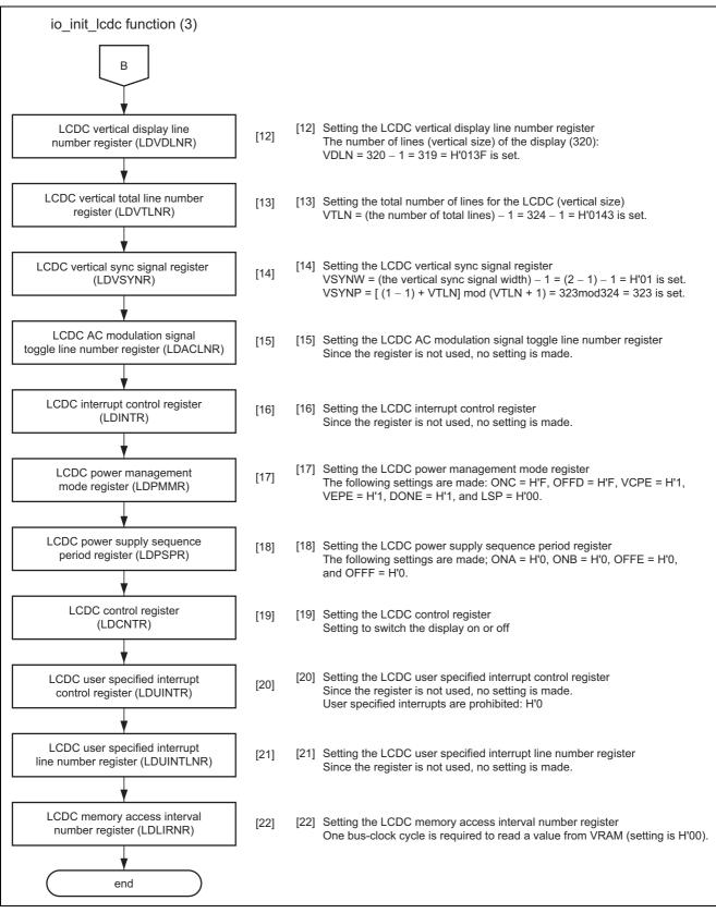
Figure 13 Flow for Initialization of the LCDC (3)
