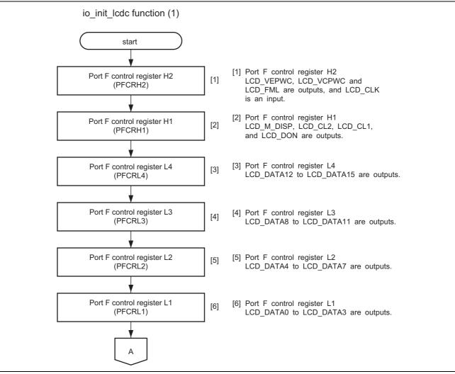
Figure 11 Flow for Initialization of the LCDC (1)
