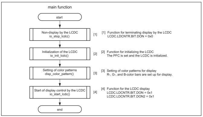
Figure 10 Flow of Processing by the "main" Function
