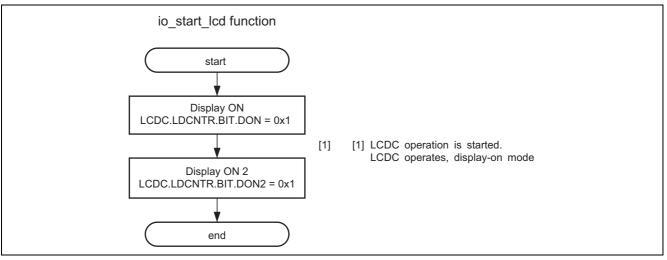
Figure 16 Flow for Starting Display Control by the LCDC
