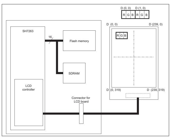
Figure 2 Hardware Configuration for the Sample Application
