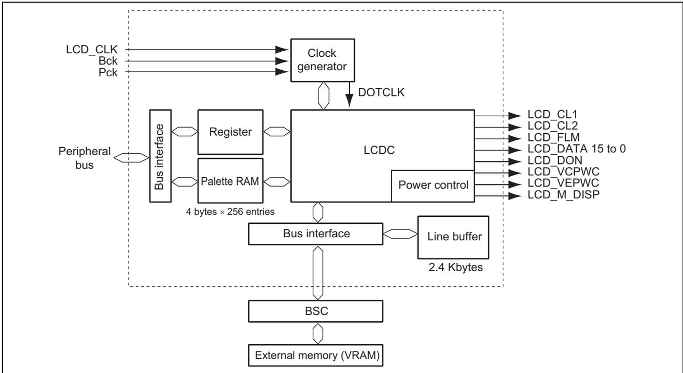
**Figure 1 LCDC Block Diagram**
