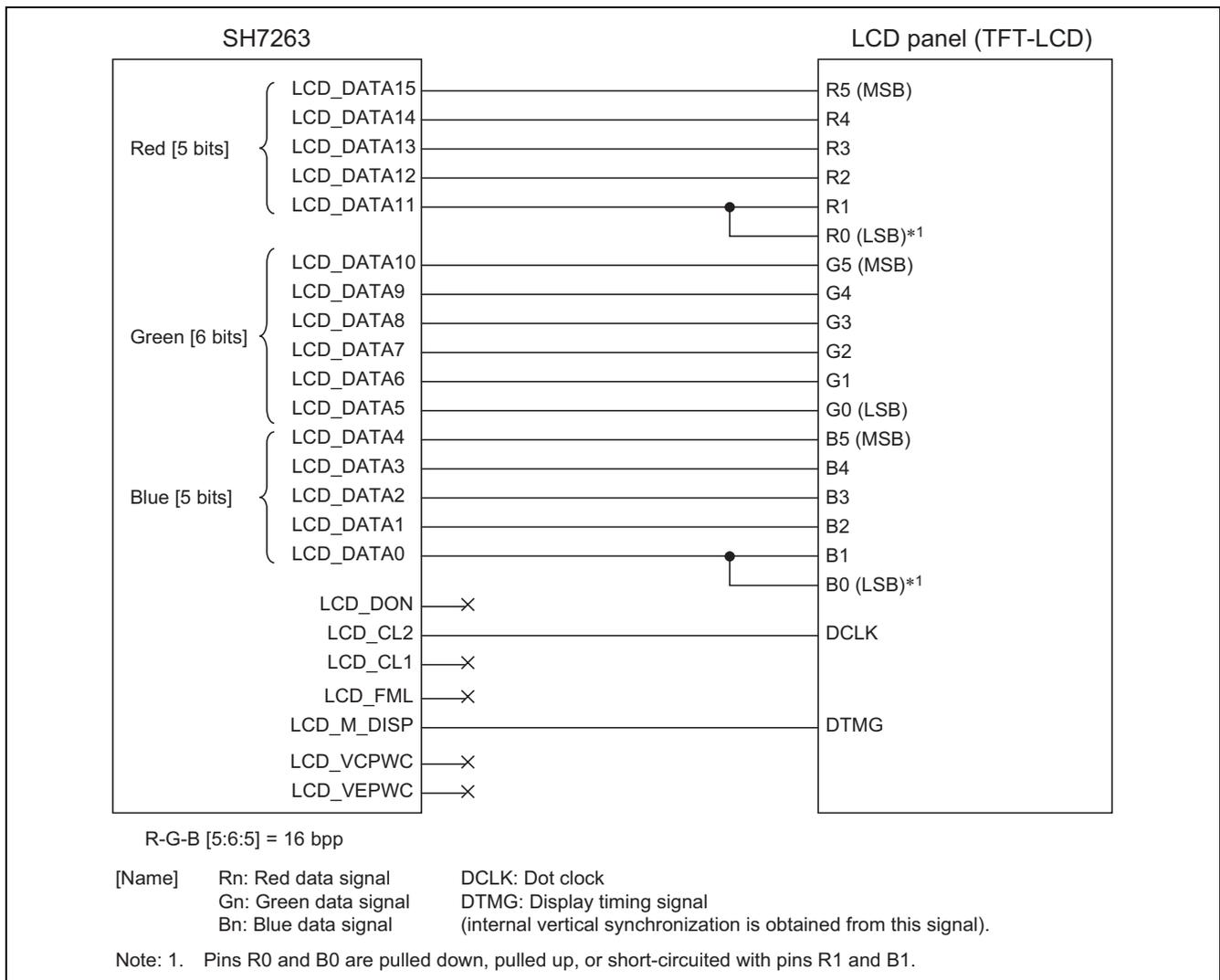
**Figure 3 Example of Connection with the LCD Panel**
