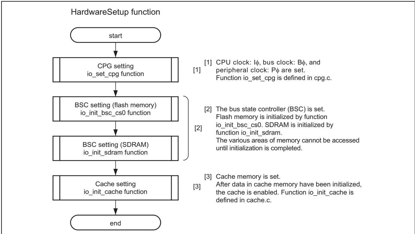
Figure 9 Flow of Processing by Hardware Initialization Function
