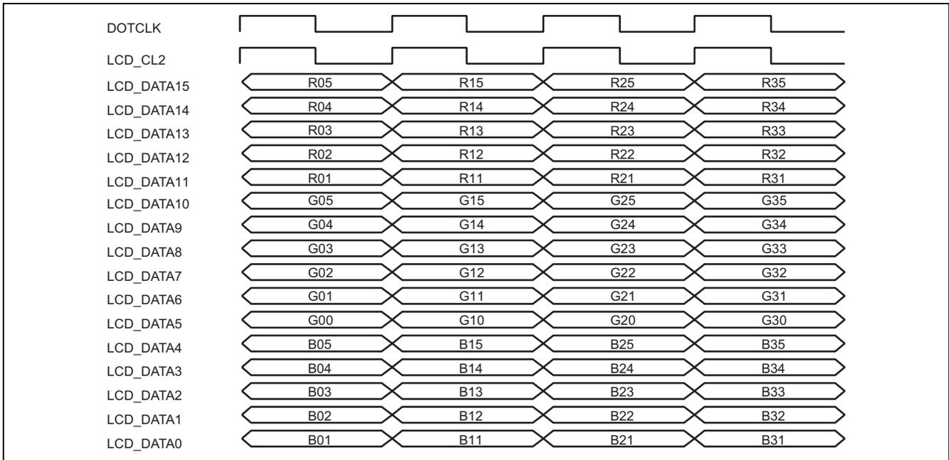
Figure 4 Example of LCD Data Signals (Color TFT Module for a 16-Bit Data Bus)
