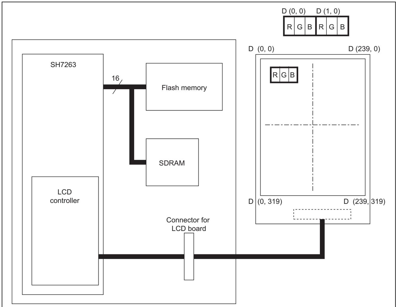
Figure 2 Hardware Configuration for the Sample Application
