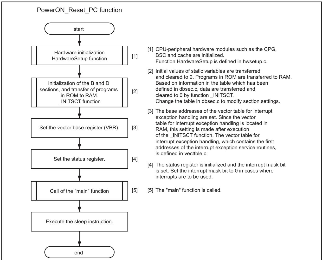
Figure 8 Flow of Processing by the Reset Program
