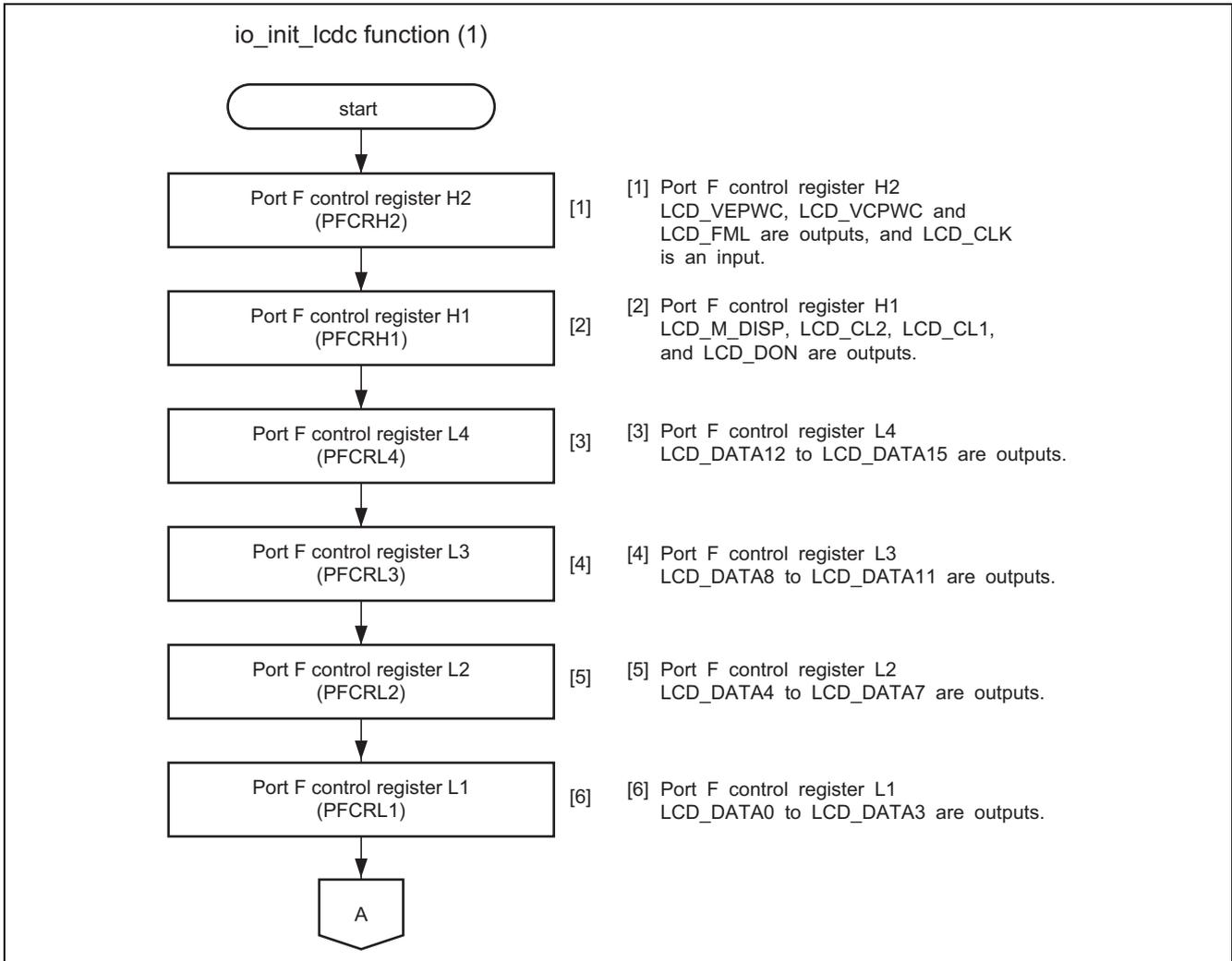
Figure 11 Flow for Initialization of the LCDC (1)
