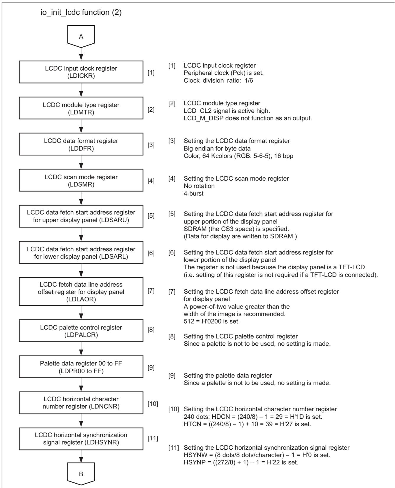
Figure 12 Flow for Initialization of the LCDC (2)
