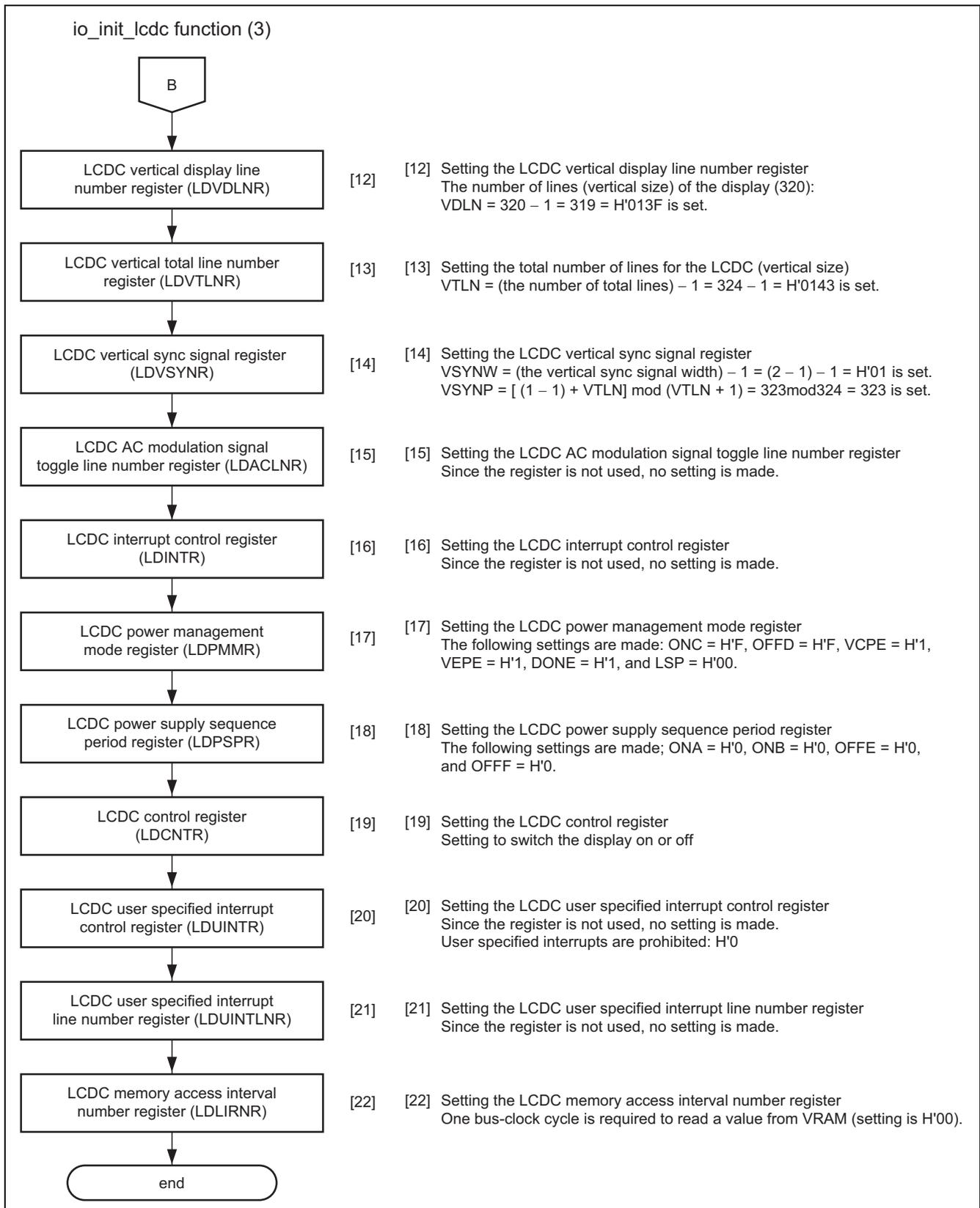
Figure 13 Flow for Initialization of the LCDC (3)
