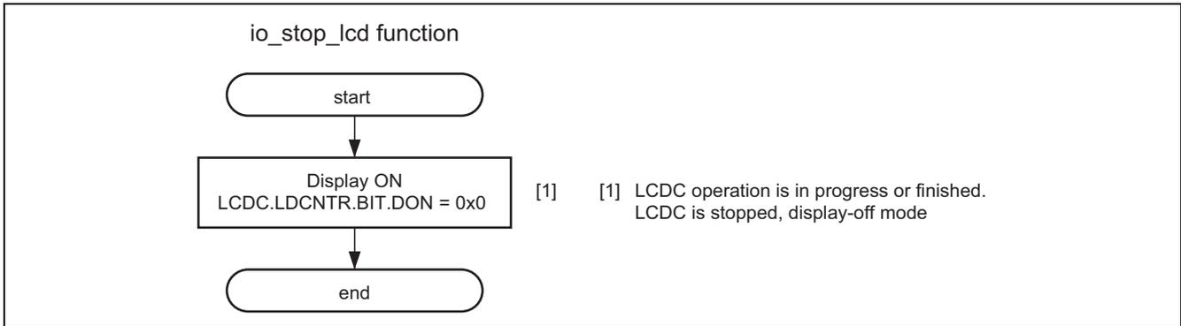
Figure 15 Flow for Terminating Display Control by the LCDC
