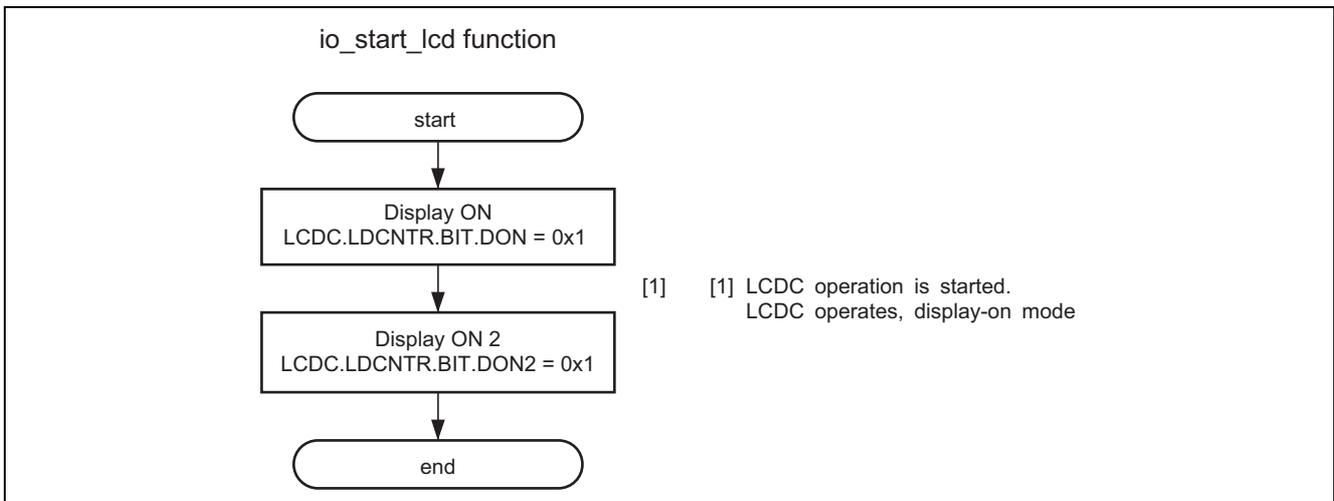
Figure 16 Flow for Starting Display Control by the LCDC
