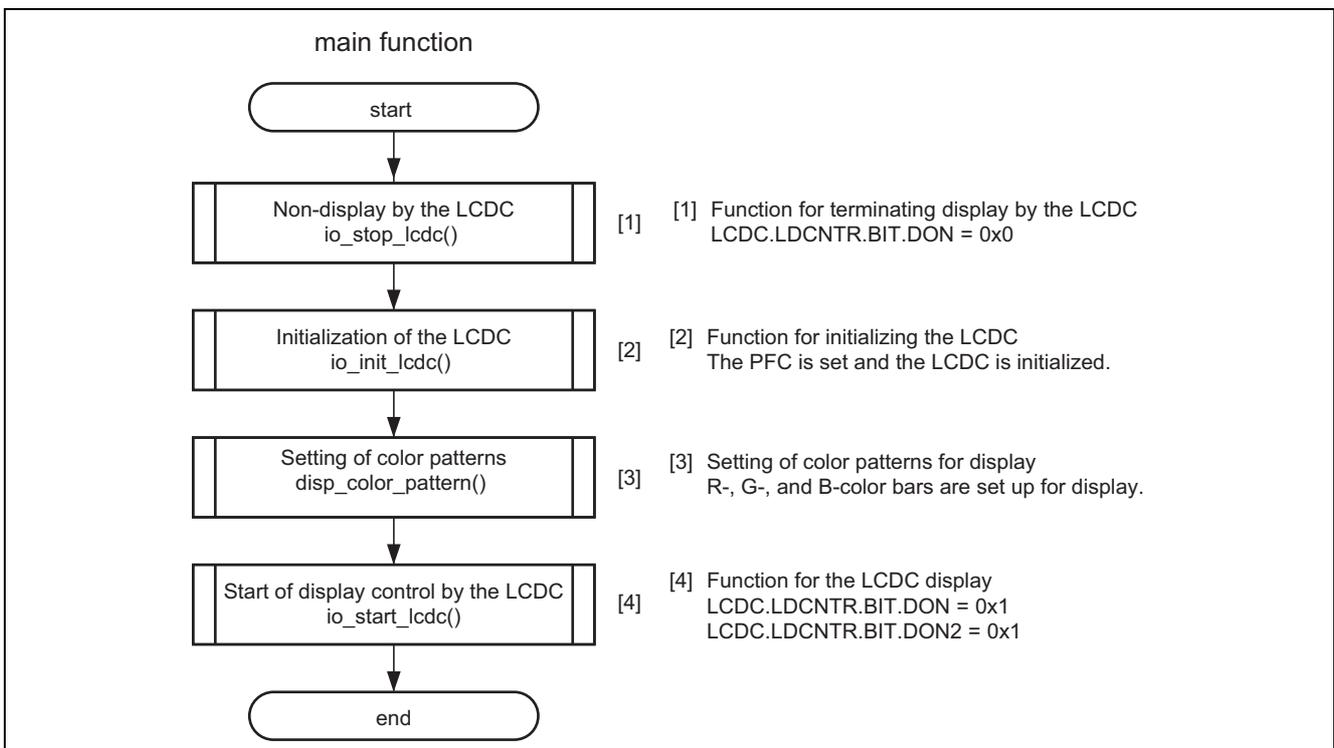
Figure 10 Flow of Processing by the “main” Function
