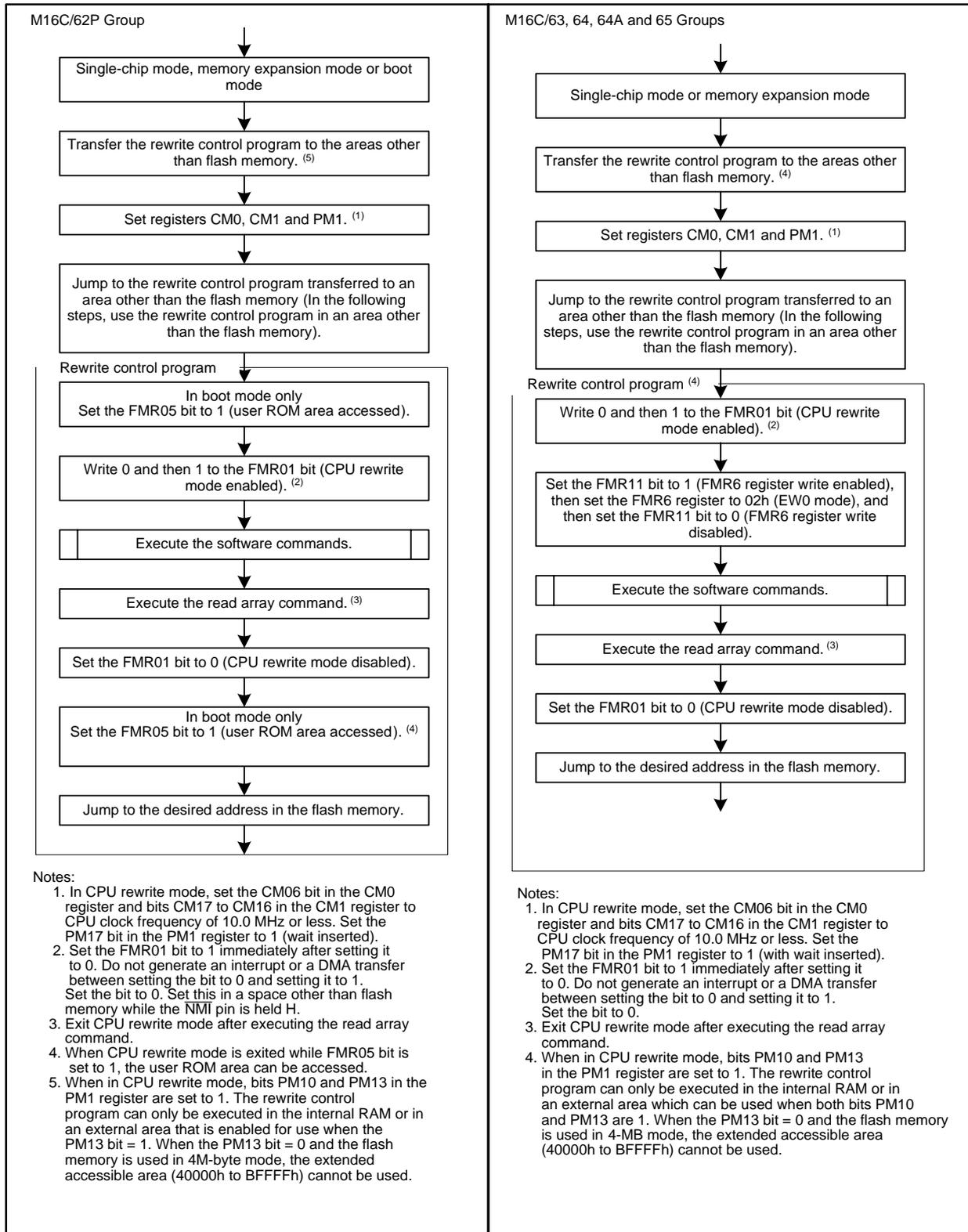
Figure 4.2 Comparison of Setting and Resetting of CPU Rewrite Mode (EW0 Mode)
