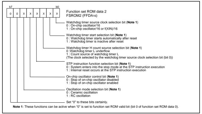
Fig. 3.3 Structure of function set ROM data 2
