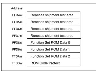
Fig.2.2 Assignment of Function set ROM area
