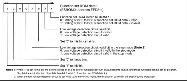
Fig. 3.1 Structure of function set ROM data 0
