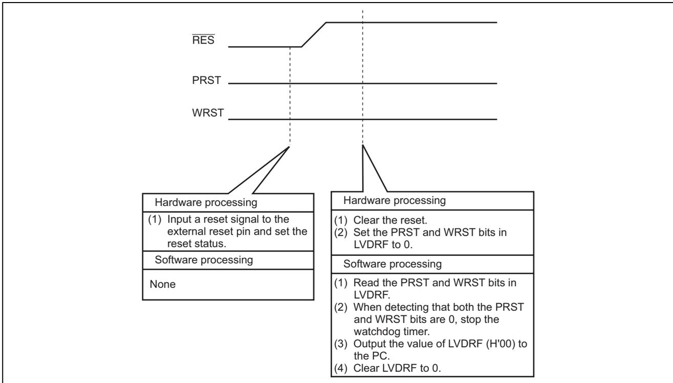
**Figure 7 Operation of a Reset by the External Reset Pin  $\overline{\text{RES}}$**
