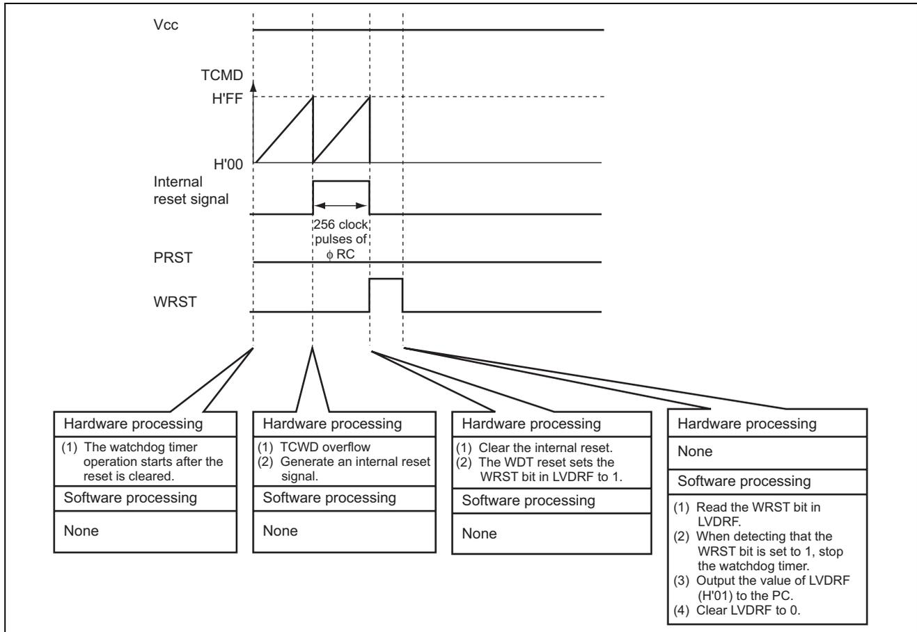
**Figure 6 Operation of a Watchdog Timer Reset**
