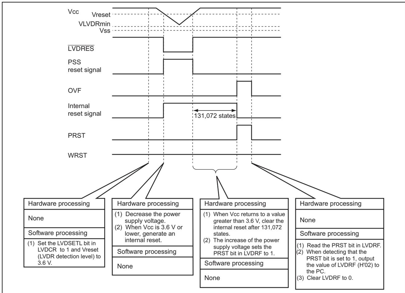
**Figure 5 Operation of the Low-Voltage Detection Reset Circuit**
