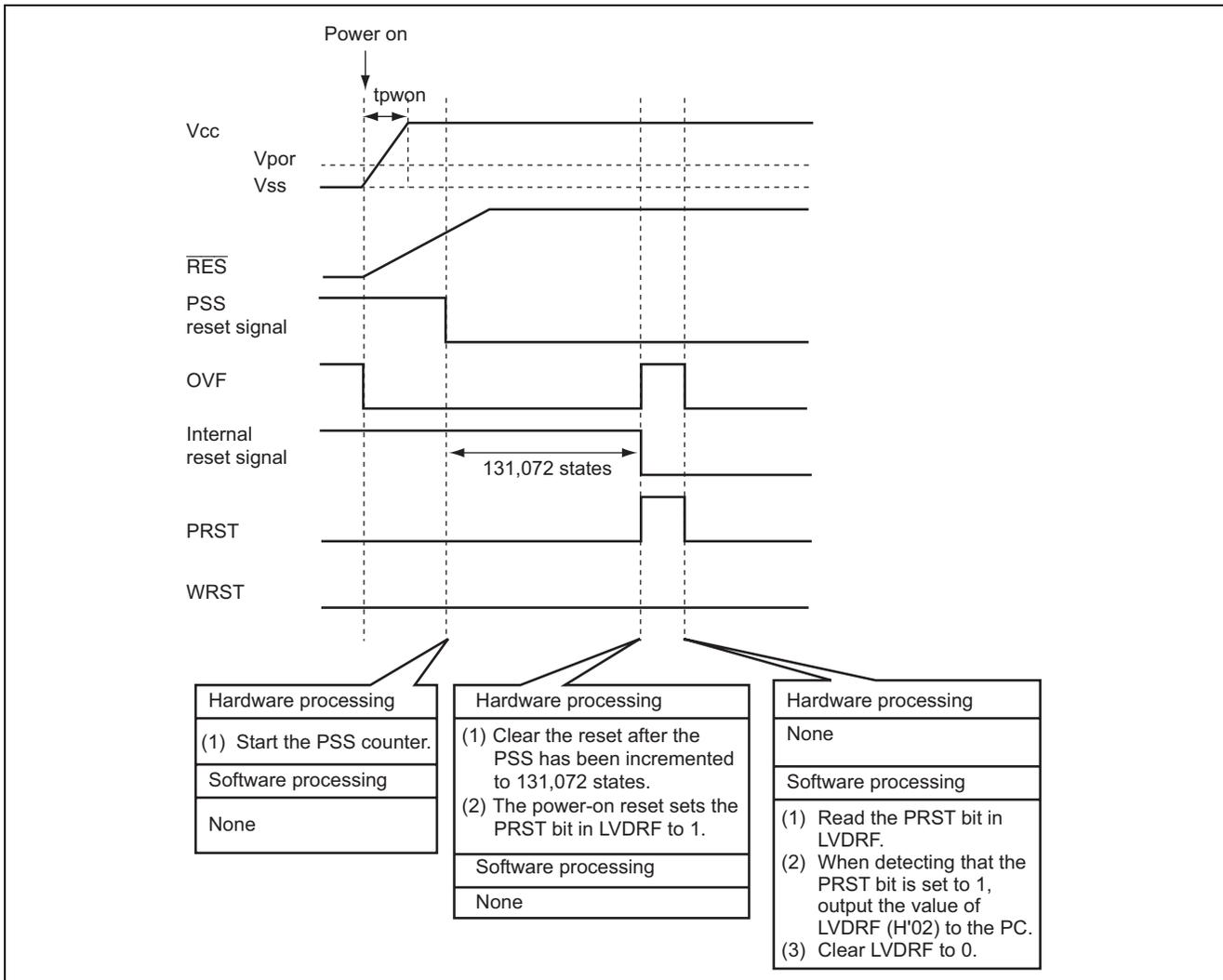
Figure 4 Operation of the Power-On Reset Circuit
