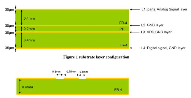
Figure 2 RF unit (50 Ohm impedance line) substrate layer configuration
