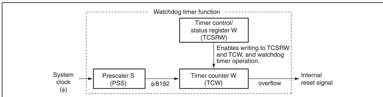
**Figure 2.1 Block Diagram of Watchdog Timer Functions**
