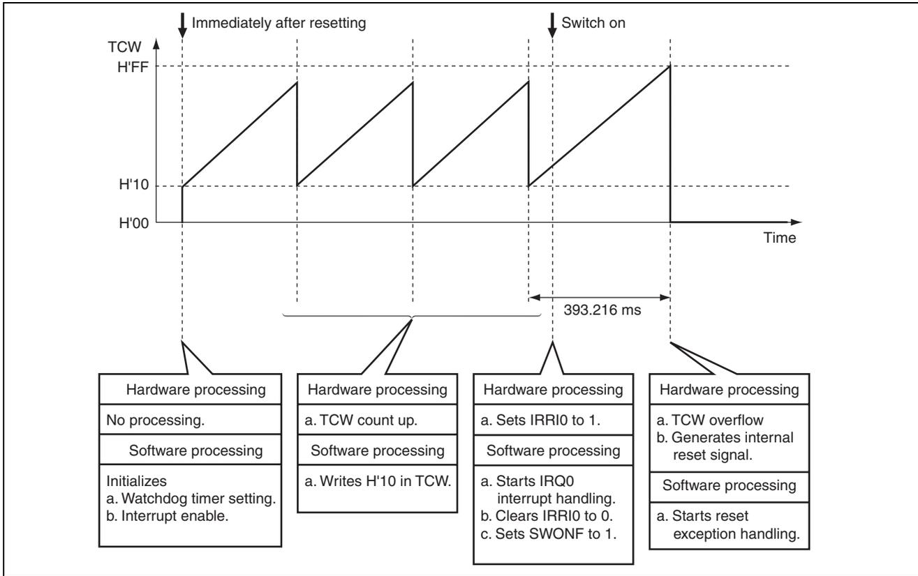
Figure 3.1 Operation Principle of Watchdog Operation by Watchdog Timer Function
