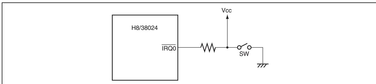
**Figure 1.1 Example of Connecting Switch to  $\overline{\text{IRQ0}}$  Input Pin**
