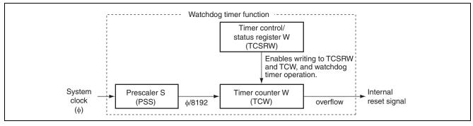
Figure 2.1 Block Diagram of Watchdog Timer Functions
