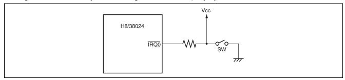
Figure 1.1 Example of Connecting Switch to IRQ0 Input Pin
