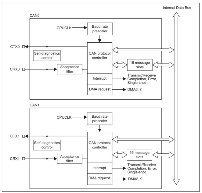
Figure 3.1.1 CAN Module Block Diagram
