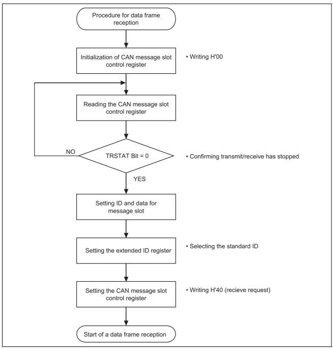
Figure 4.3.1 Data Frame Reception Processing
