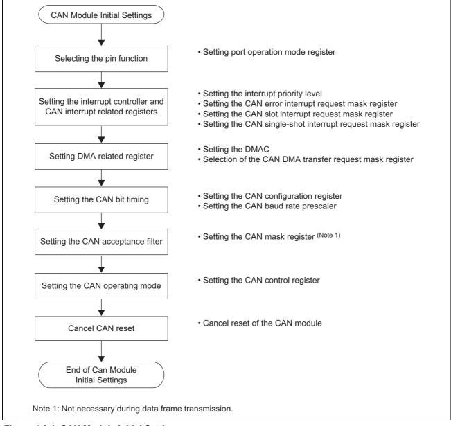
Figure 4.2.1 CAN Module Initial Setting
